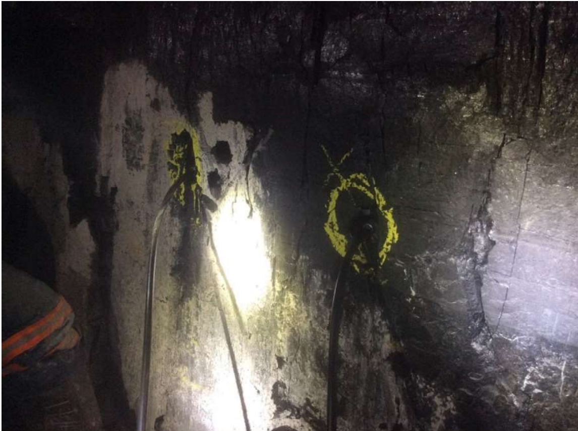
Figure 3.7: The two extensometers installed in the cross-cut. The heads were ultimately fixed to the borehole mouth using wooden wedges.
