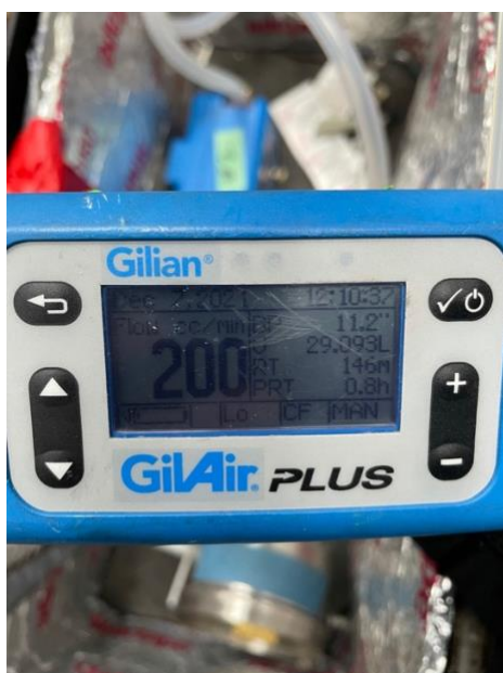
Figure II-4. Blue GilAir Plus Sampling pump at 200mL/min
