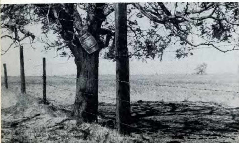
Mosquito Control at International Airports. In flat, dry pastures a nail keg was used for a mosquito collecting station.
