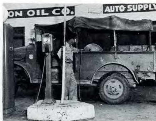
The 50-gallon air tank, which furnished compressed air for the spray cans, was filled at service stations.
