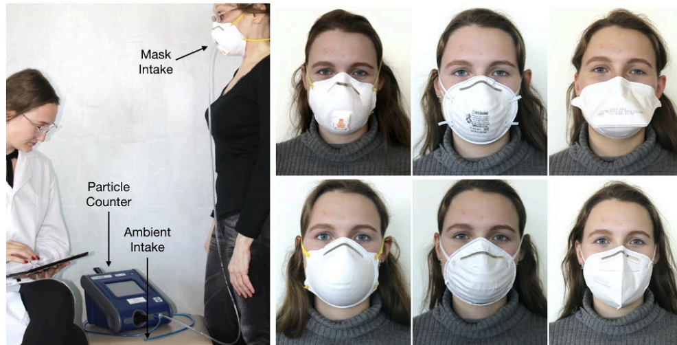
Figure 15. Quantitative fit testing setup with N95 and KN95 samples worn by one of the participants [63]
