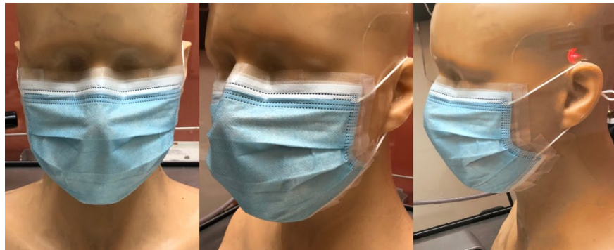
Figure 22. Sealing the surgical style mask to the animatronic headform
