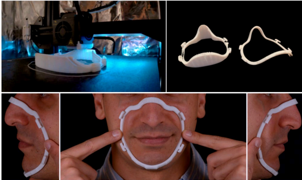
Figure 17. 3D printed mask fitter using face scanning technology [70]
