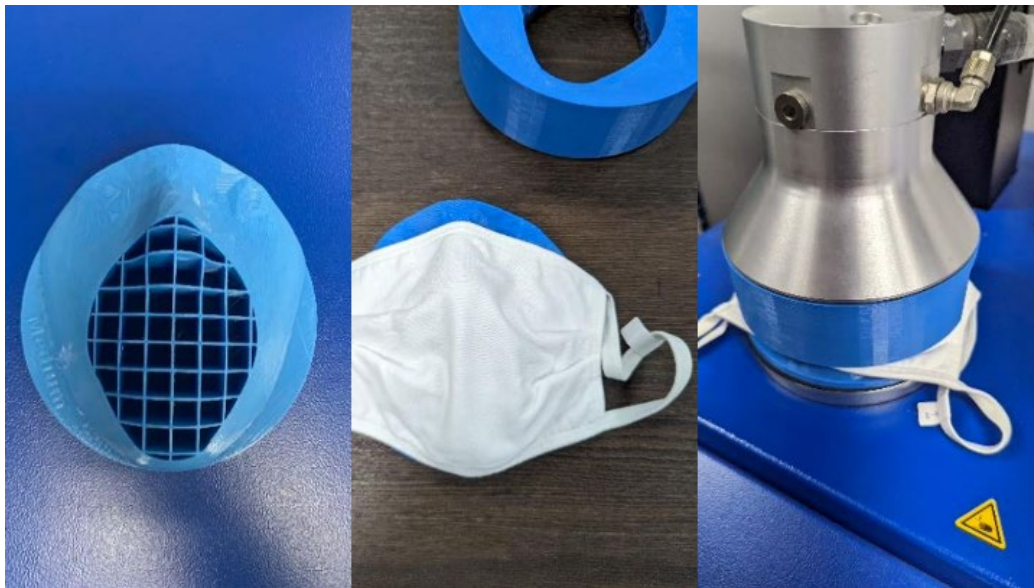
Figure 36. ASTM F3502-21 Standard Specification testing with the printed adult medium face form (left), mounted sample (middle), and test setup (left) from Intertek
