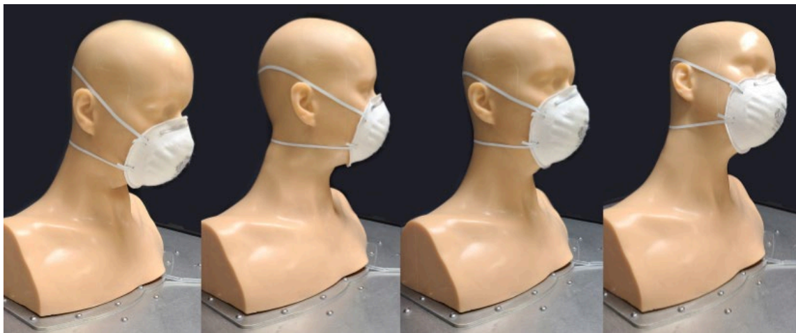
Figure 21. Headform movements from left to right: head nod up and down, head shake side to side, jaw bite opened and closed, and head wobble shoulder to shoulder
