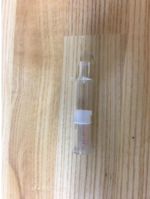
Figure A.8. Modified OVS Tube with Resin Removed for the Particle-Phase Efficiency Trials
