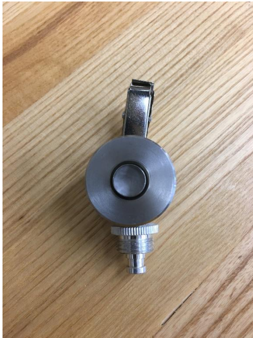
Figure A.9. Modified IFV Pro (IFV Pro Head Without Sorbent Tube) for the Particle-Phase Efficiency Trials
