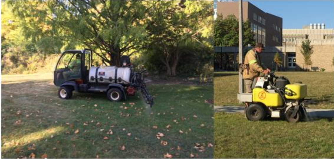
Figure A.12. Subject 1 (Company A) Applying Dicamba and MCPA to Fields Using a Toro Multi-Pro® Turf Sprayer and a Z-Spray Stand-On® Sprayer
