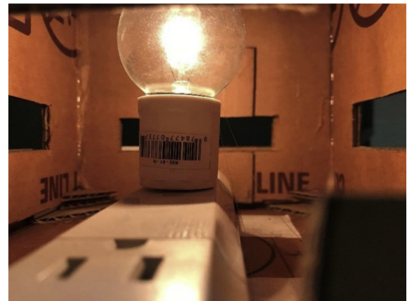
Fig. 3. Incandescent bulb placed in tower. Note surrounding slits that facilitate free convection.
