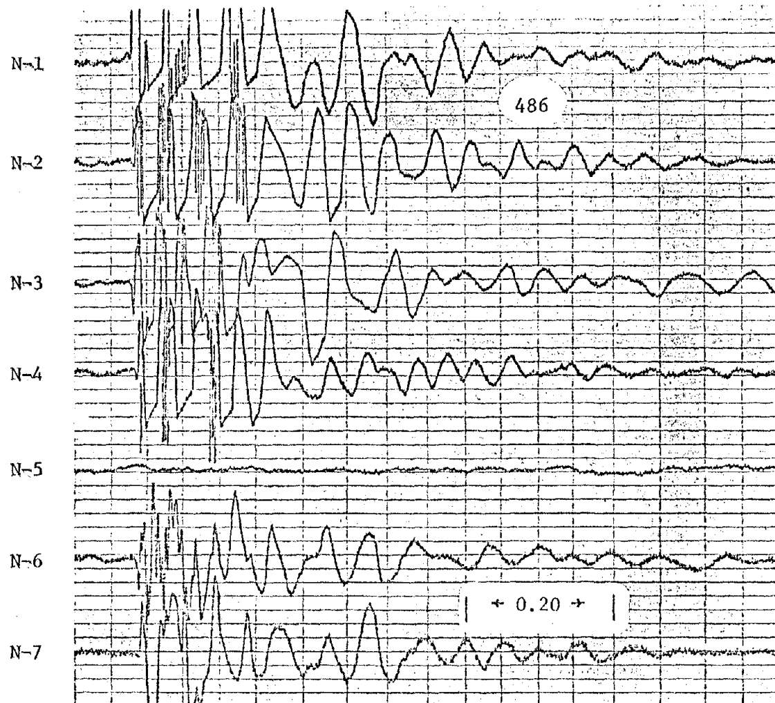
Figure 45. Event (38-3854), February 26, 1974, "Medium Caving." [Horizontal Scale: Time (s); Vertical Scale: Particle Velocity ( \mu ips/10 divisions).]
