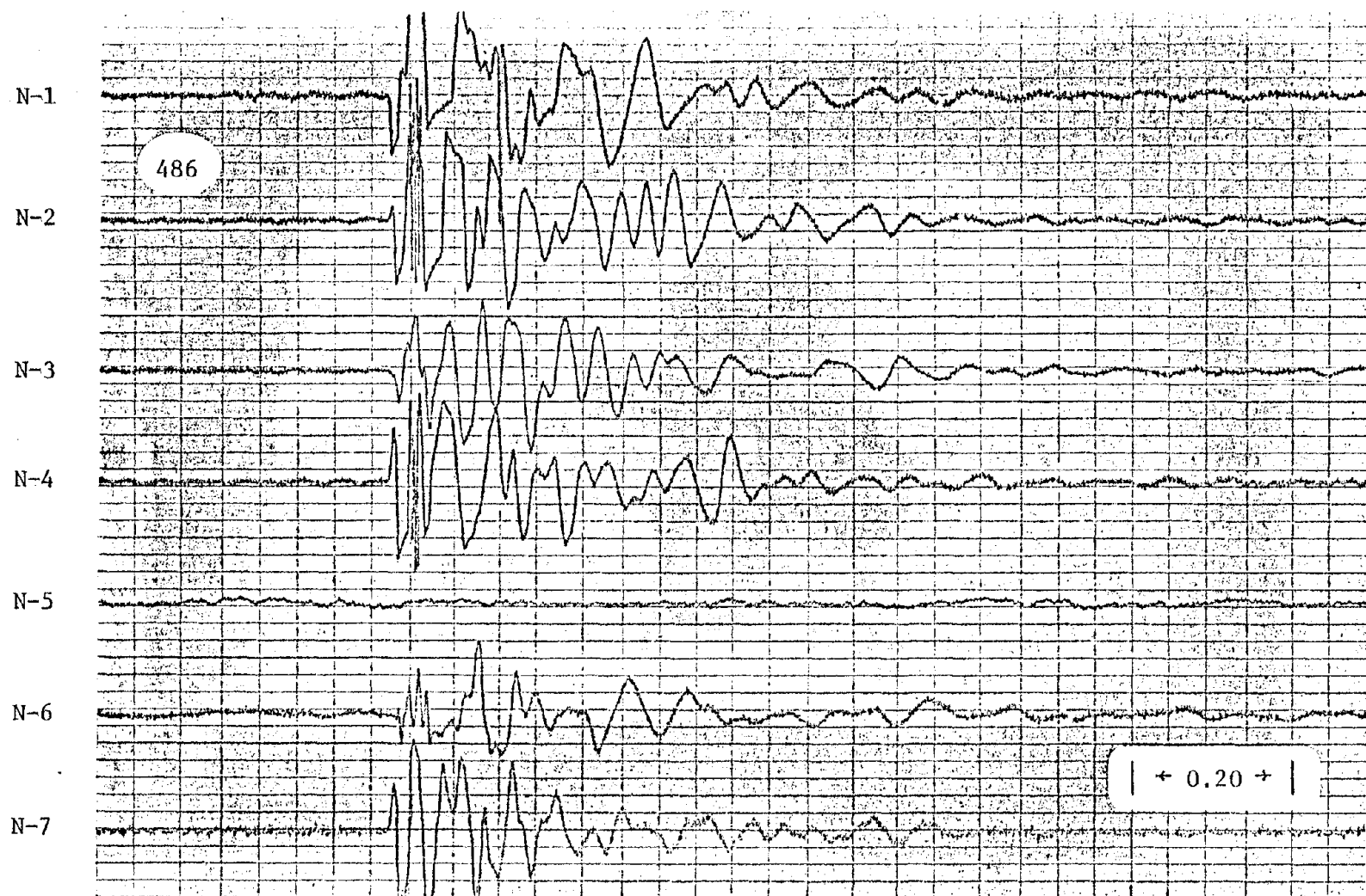
Figure 38. Event (38-4894), February 26, 1974--Time-Expanded. [Horizontal Scale: Time (s); Vertical Scale: Particle Velocity (pips/10 divisions).]
