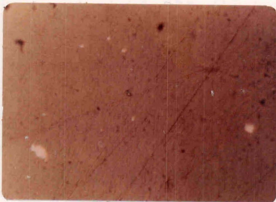
Figure 18. Tiny, irregularly shaped goethite grains, 1-10 \mu\text{m} across, disseminated in bauxite. Such grains are commonly scattered throughout ferruginous bauxites.
