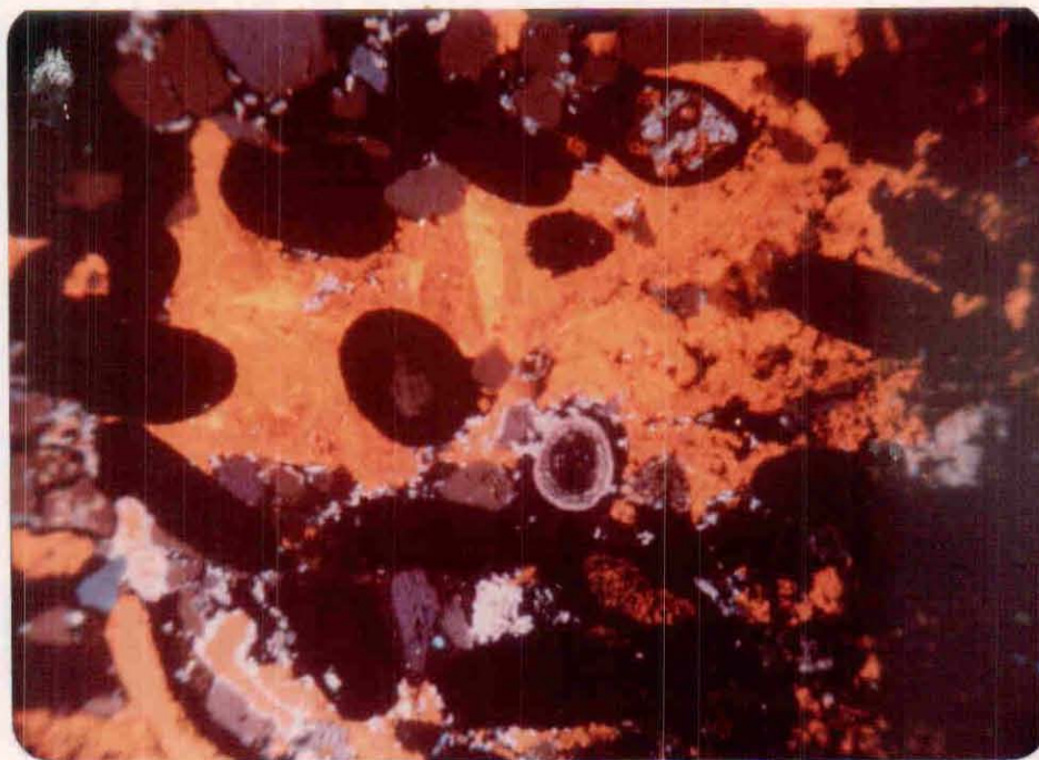
Figure 10. Luminoscope micrograph showing a collophane ring (light purple) in a hematite oolite together with many tiny disseminated collophane grains (light blue luminescence) mostly contained in hematite (black) but partly in calcite (orange).
