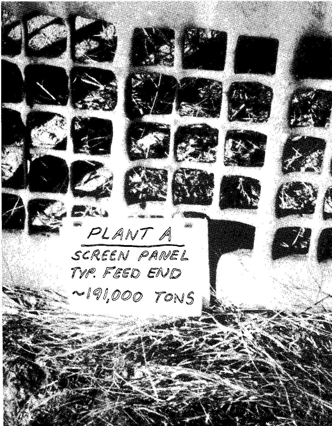
FIGURE ES-11 - Plant A - resilient top screen deck after processing 191,000 tons.
