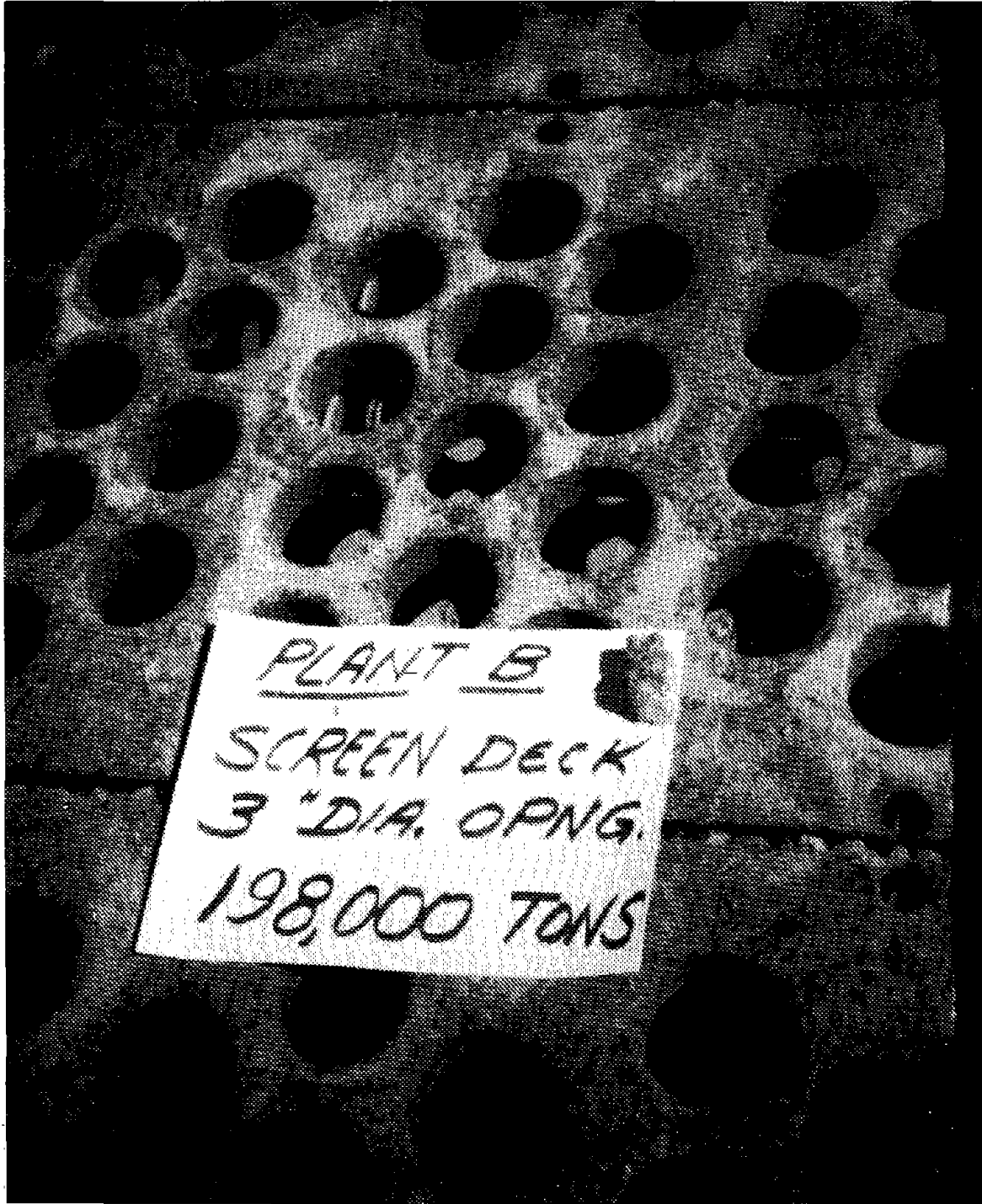
FIGURE ES-5. - Plant B - resilient screen deck after processing 198,000 tons.
