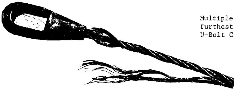
Multiple strand breaks inside or at the base of the socket on a Zinc Poured Socket WRT.
