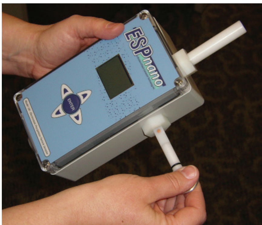
Figure 1: Inserting a “sampling key” into the ESPnano model 100 particle sampler. During operation, particles enter the device via the white inlet tube at the top of the sampler.
