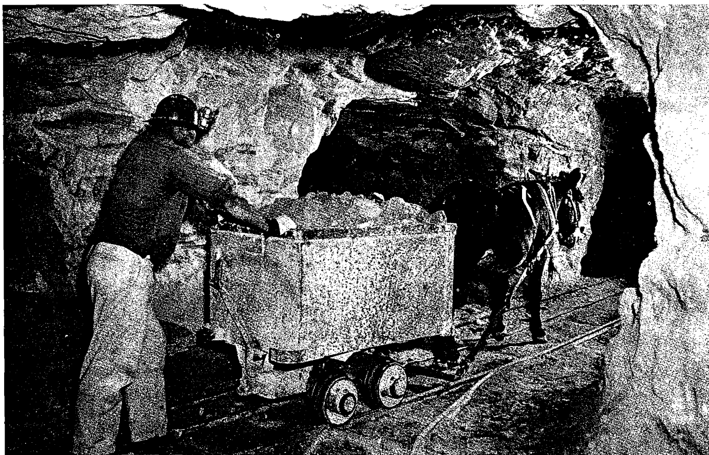
FIGURE 21. - Burro Haulage in Frank No. 1 North Adit.
