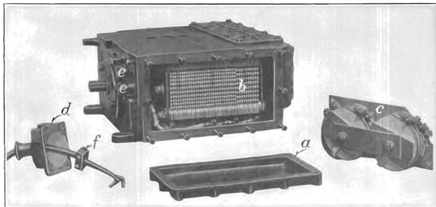
B. JEFFREY 35B DIRECT-CURRENT MACHINE, RHEOSTAT COMPARTMENT OPEN FOR INSPECTION.
