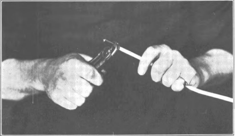
A. CRIMPING DETONATOR ON FUSE.
