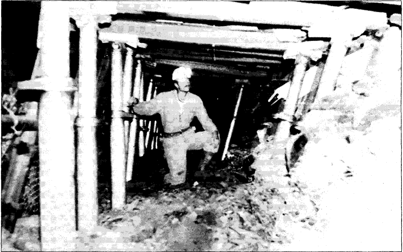
Fifth Left tailgate entry during panel 5 mining. Hydraulic supports have been used to reinforce yieldable steel sets against front abutment loading from nearby approaching face; wire mesh was utilized to prevent infilling of escape walkway by loose material from rib sloughage and minor roof falls.
