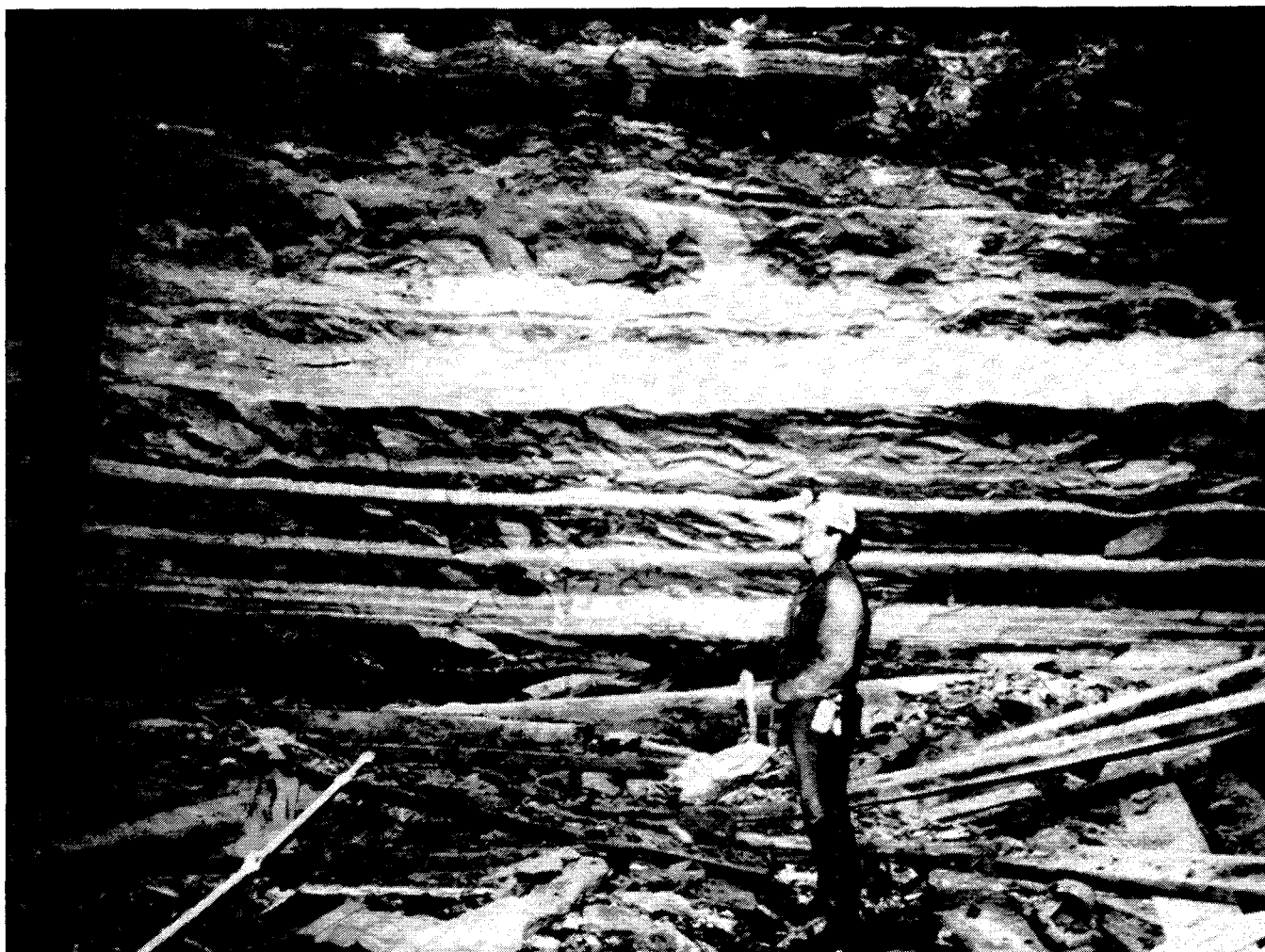
Castle Gate No. 3 Mine roof strata exposed at shaft station in north side of mine. Large slabs of thinly bedded sandstone, siltstone, and mudstone separate along bedding planes, leading to roof falls.
