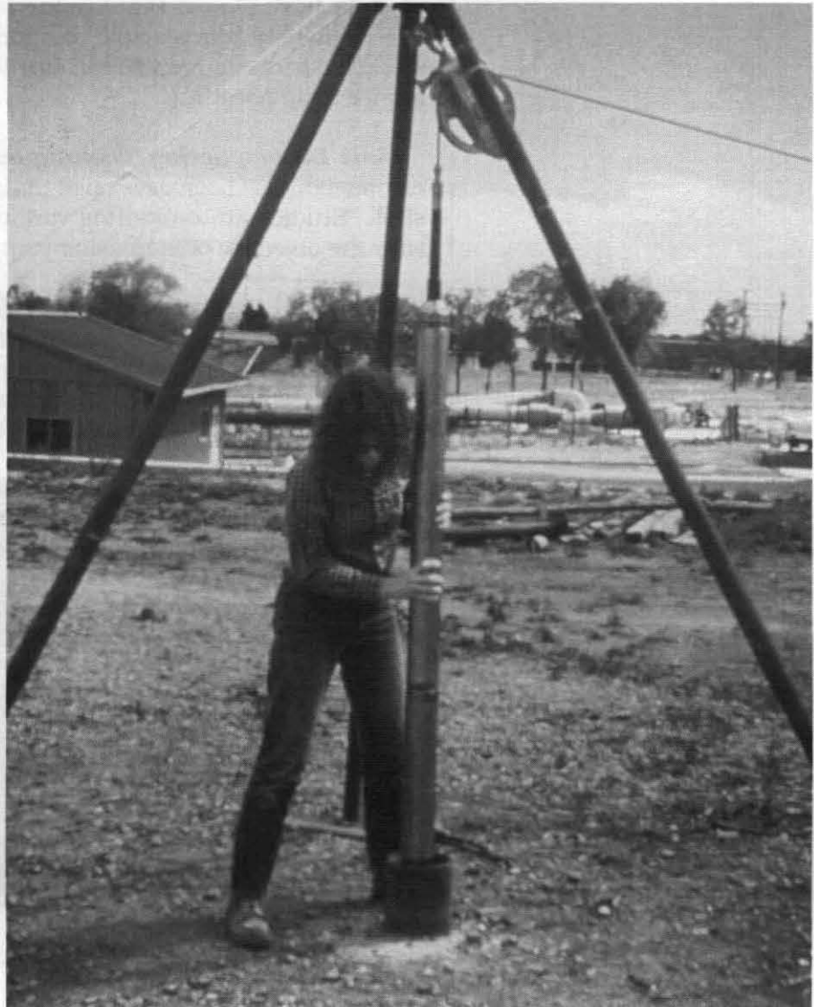
Field tests of a cross well acoustic tomography system to locate abandoned underground mines and subsidence failure.
