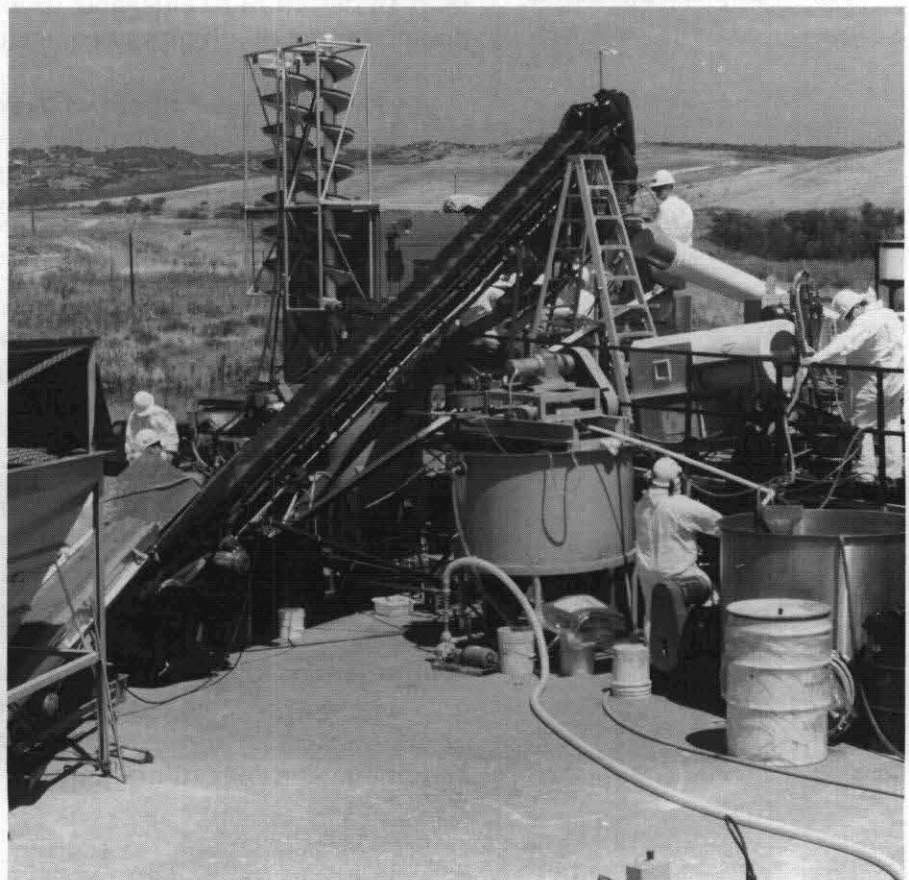
Demonstration of USBM-developed technology at Camp Pendleton, CA. USBM and Navy personnel are operating the gravity circuit of a process plant for removal of lead bullet fragments and lead in soil at small-arms firing range.
