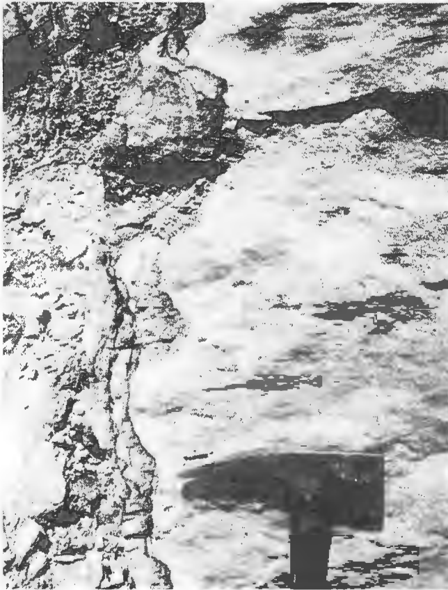
Figure 3.—Close-up of incipient weathering and parallel fracture development adjacent to stress-relief joint in massive sandstone.
