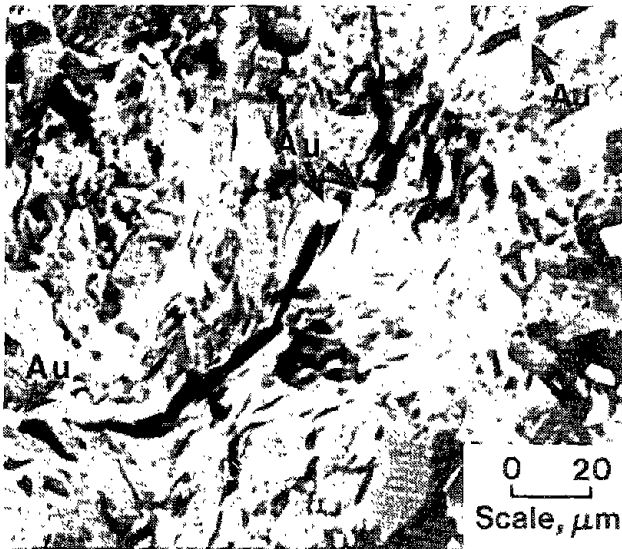
Figure 2.—BEI showing four Au grains in open fracture of schist from Cyprus Copperstone Mine. [From Blake and Earley (11)].
