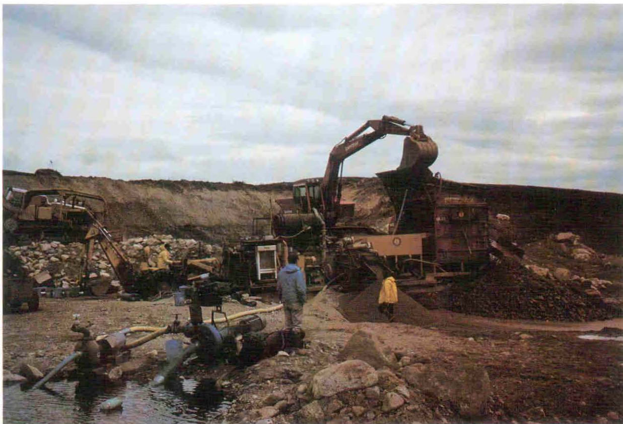
FIGURE 11.- Mining operation on Busch Creek showing the jig plant gold recovery system.
