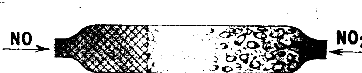
FIGURE 6. - Schematic of nitrogen oxides detection tube, by aspirating from right to left \text{NO}_2 is indicated, when aspirated from left to right the sample passes over the oxidizer and \text{NO}_x is indicated.
