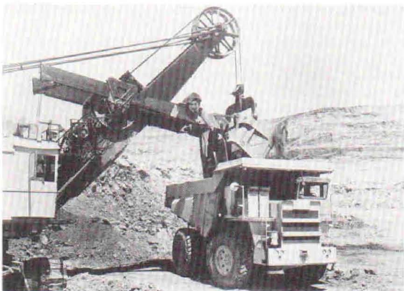
A 9-cubic-yard shovel loads borate ore into a 50-ton truck in an open pit mine on the Mojave Desert near Boron, Calif. The ore is hauled to an automatic 1,300-foot conveyor that carries it to processing plants on the surface. (Courtesy of U.S. Borax and Chemical Corp.)
