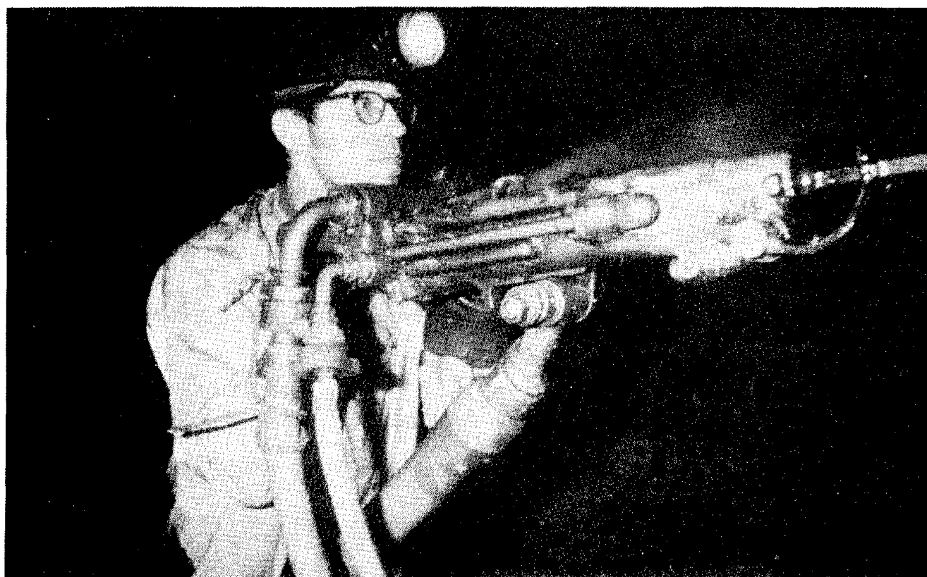
Figure 2.—The jackleg drill is used in a variety of angles in underground metal-nonmetal mines.
