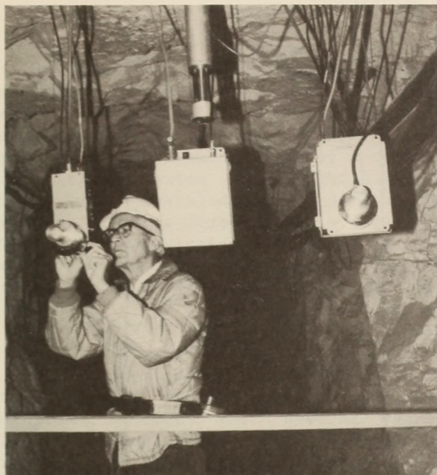
FIGURE 16. - Two model B-100 CWL detectors equipped with Zeleny tubes. Detector on right contains a charged wire.
