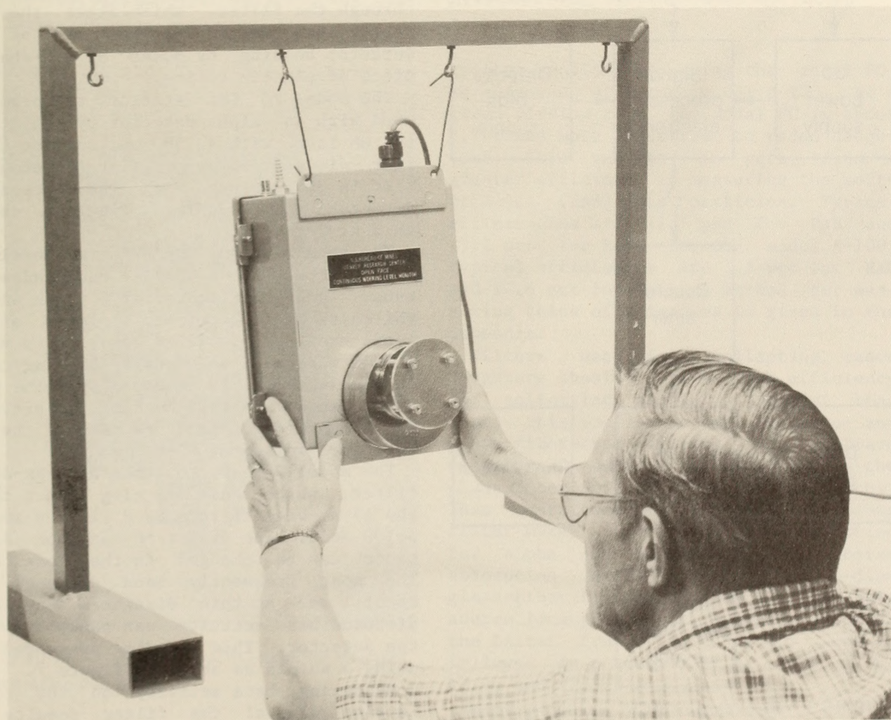
FIGURE 2. - Model B-100 CWL detector mounted on metal enclosure for associated electronics, with beta shield.
