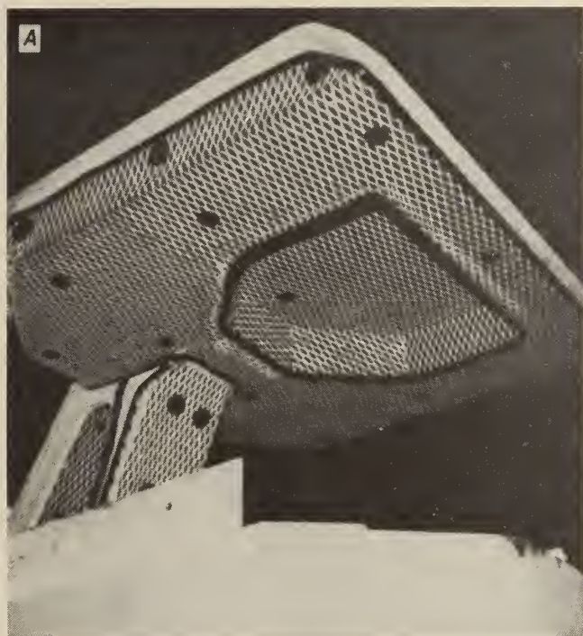
FIGURE 45. - LHD operator-compartment noise-control treatments. A , Canopy; B , foot-pedal area.
