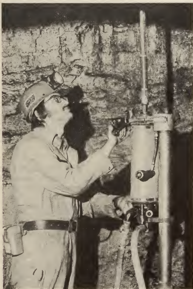
FIGURE 28. - Stoper with retrofit noise-control treatments in operation.
