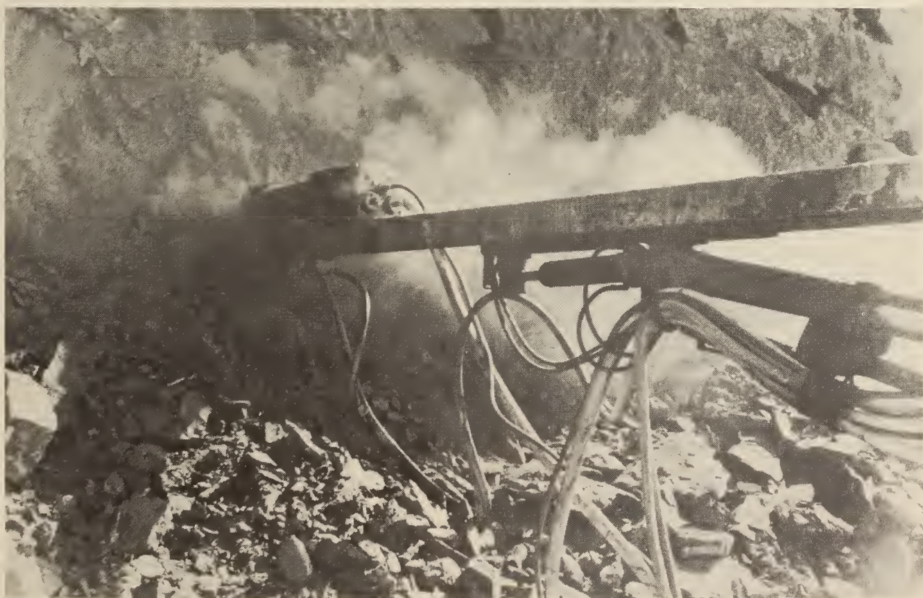
FIGURE 39. - Redesigned, noise-controlled jumbo drill at completion of hole.
