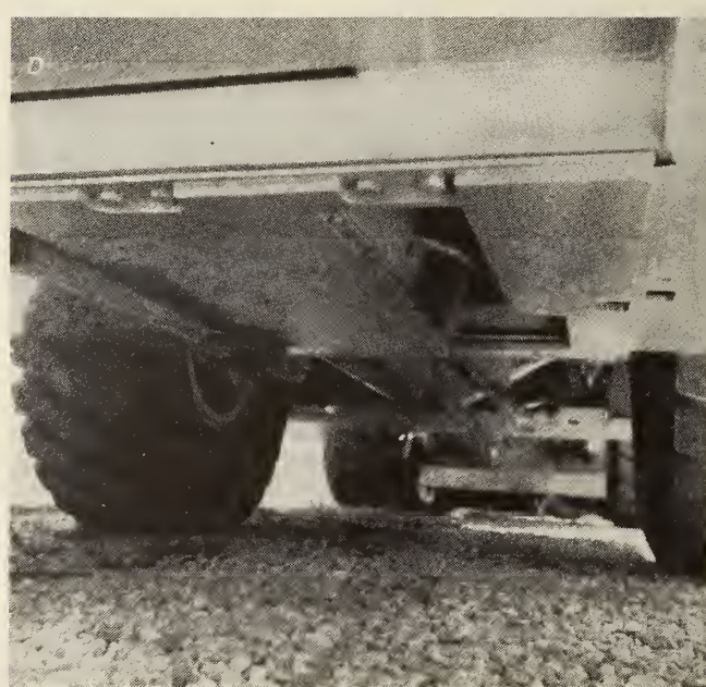
FIGURE 42. - Retrofit acoustical enclosure for LHD engine. A , Top cover; B , right side cover; C , left side cover; D , belly pan treatment.
