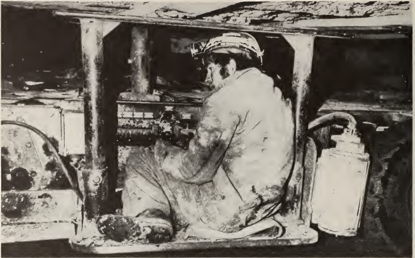
FIGURE 17. - Operator cramped within tram compartment on cutting machine.
