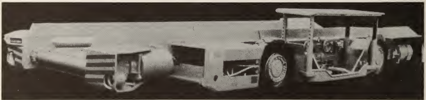
FIGURE 8. - Center-mounted cab and canopy on Joy shuttle car.
