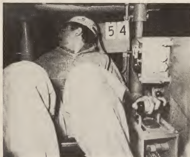
FIGURE 16. - Operator under 35-in canopy tramming outby.
