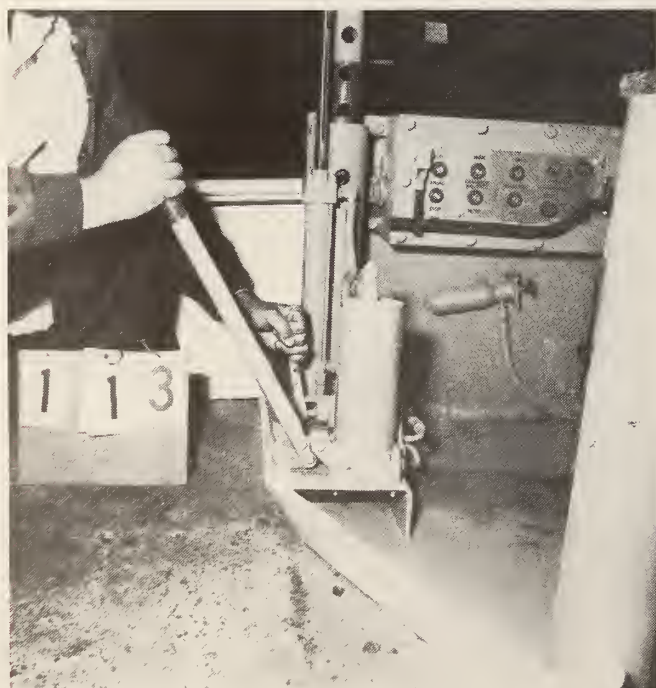
FIGURE 8. - Operating the canopy adjusting pump and flow valve.
