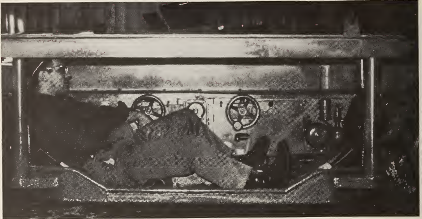
FIGURE 1. - Rib-reinforced canopy on Joy shuttle car.
