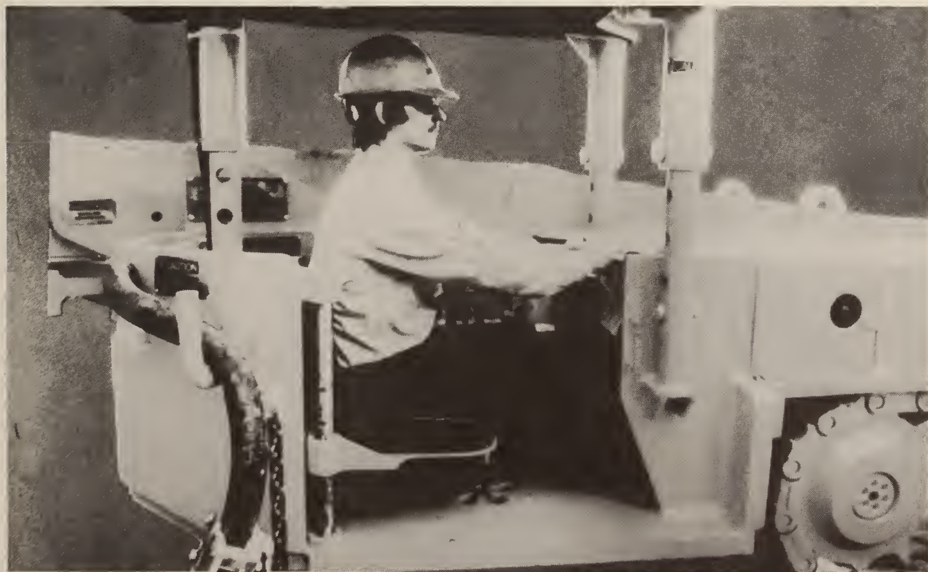
FIGURE 6. • Prototype cab and canopy on LN 800 continuous miner.
