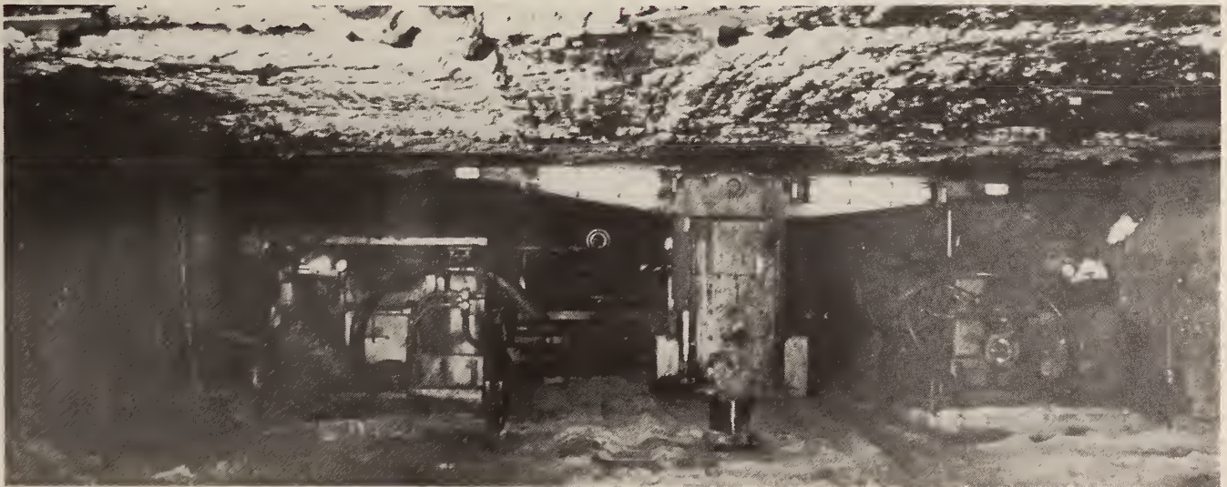
FIGURE 16. - Dual operator stations at front of dual-head roof bolter.
