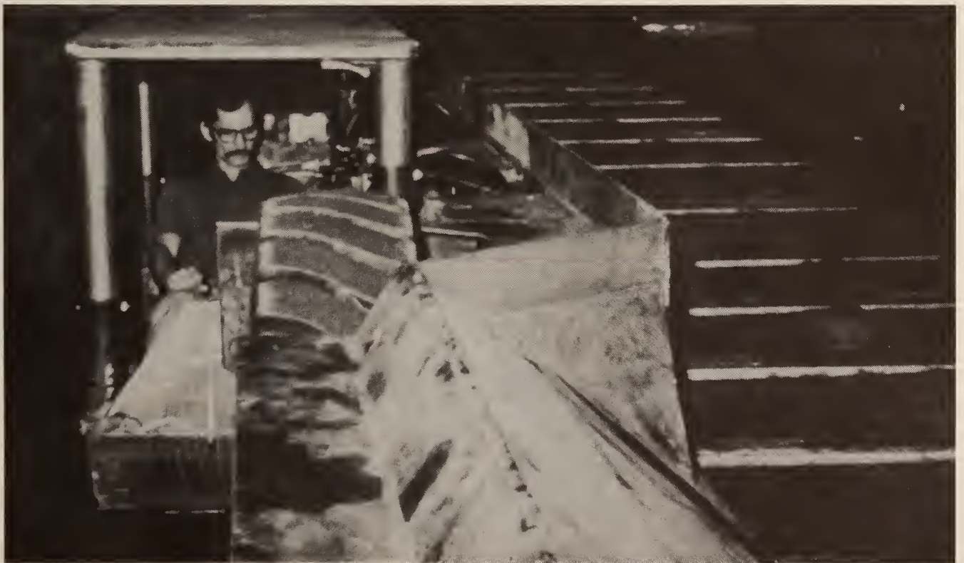
FIGURE 11. - Modified floating cab on center-driven shuttle car (end view).
