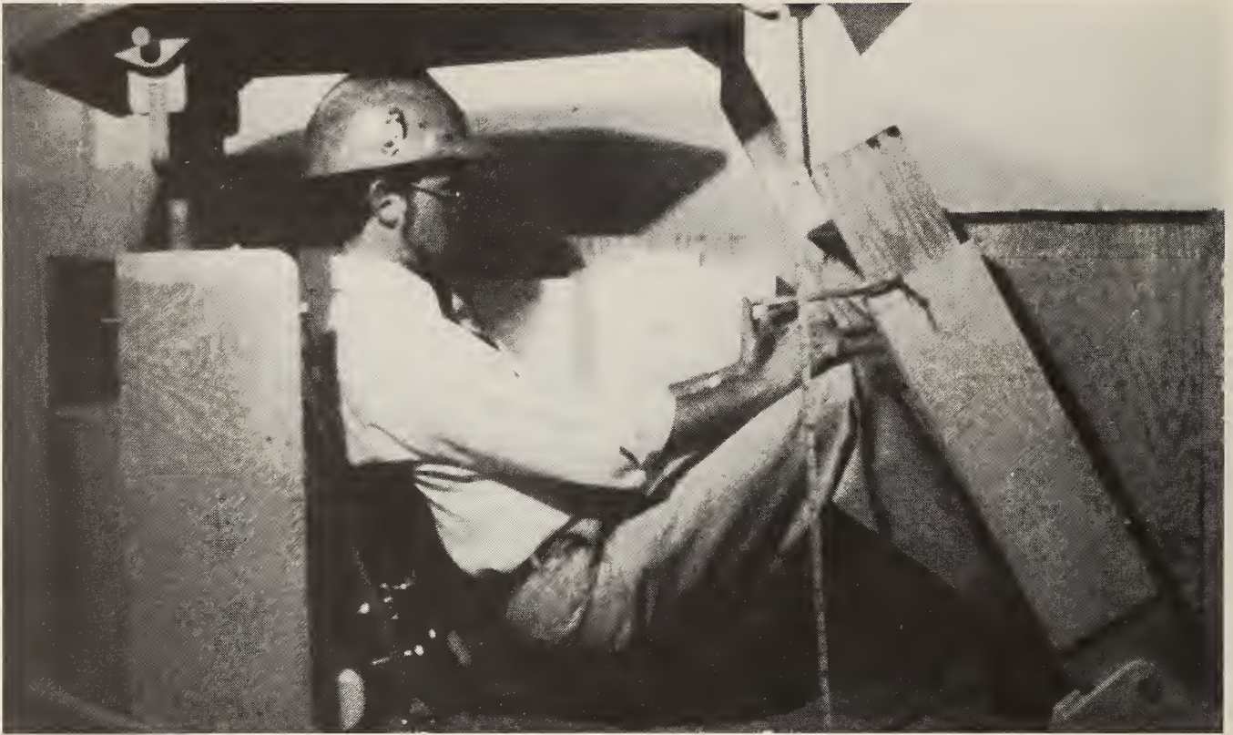
FIGURE 2. • Cab mockup - 50th percentile operator with canopy in low position.
