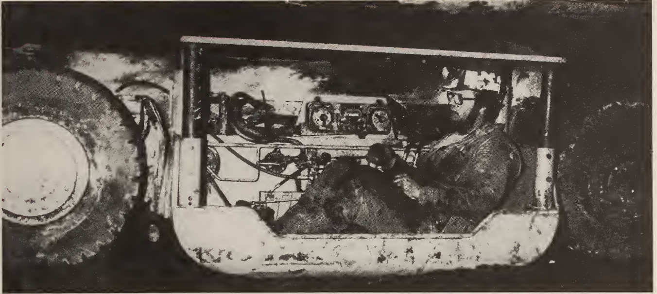
FIGURE 4. - Floating operator's deck on center-driven shuttle car.
