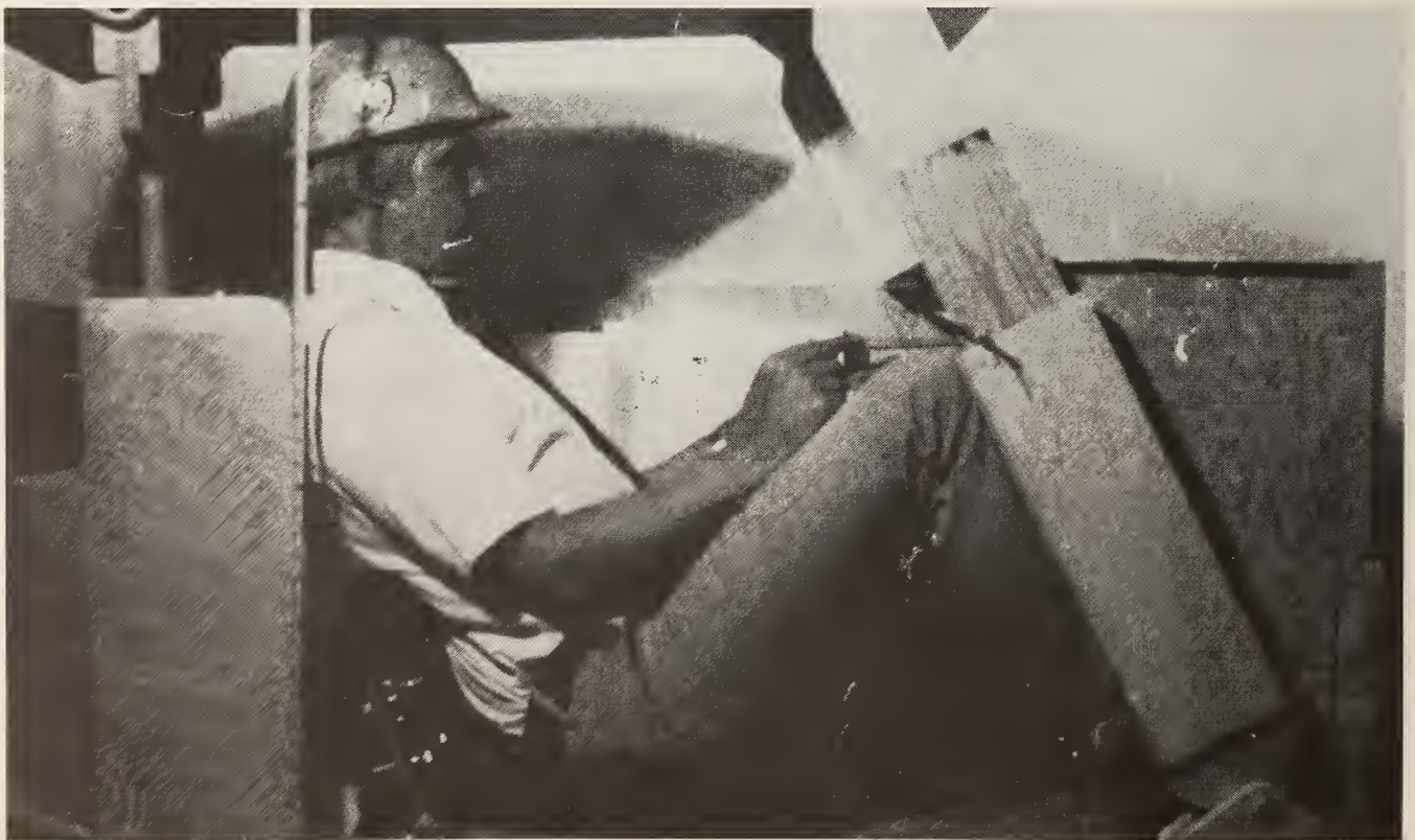
FIGURE 3. • Cab mockup - 95th percentile operator with canopy in low position.
