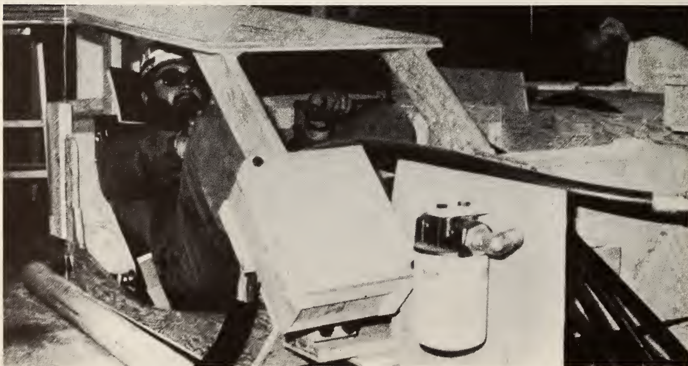
FIGURE 6. - Wooden mockup used to design continuous miner cabs.
