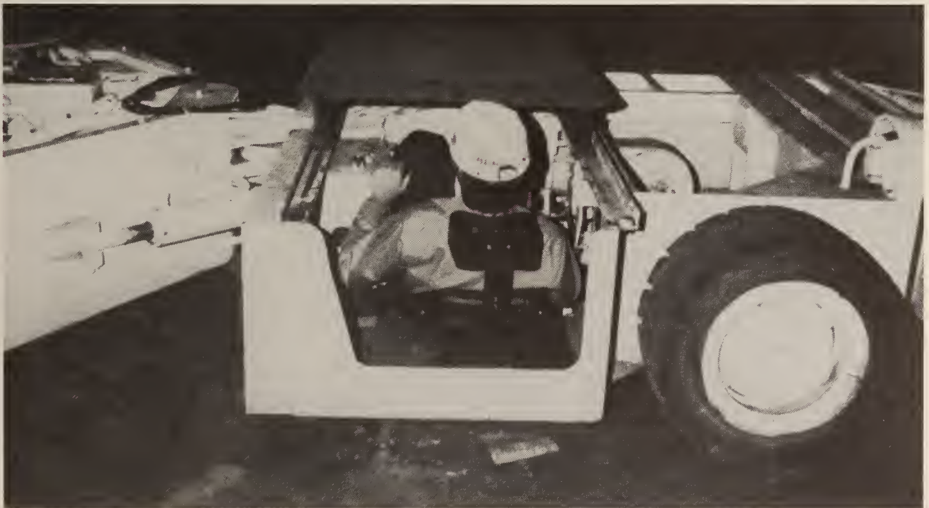
FIGURE 10. - Sliding canopy top on scoop for easier ingress and egress.
