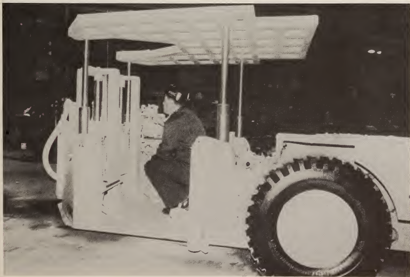
FIGURE 3. - Model 370 roof bolter with central operator platform and canopy.
