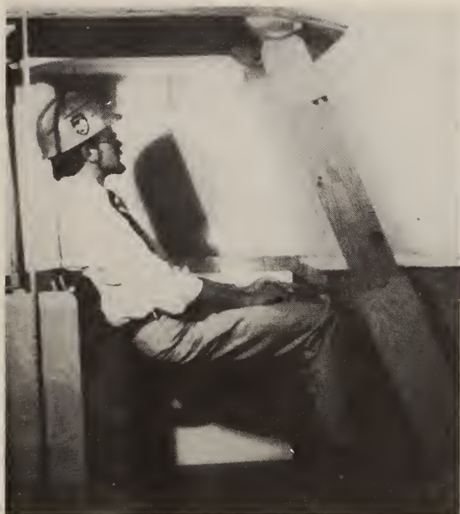
FIGURE 4. • Cab mockup - 50th percentile operator with canopy in high position.
