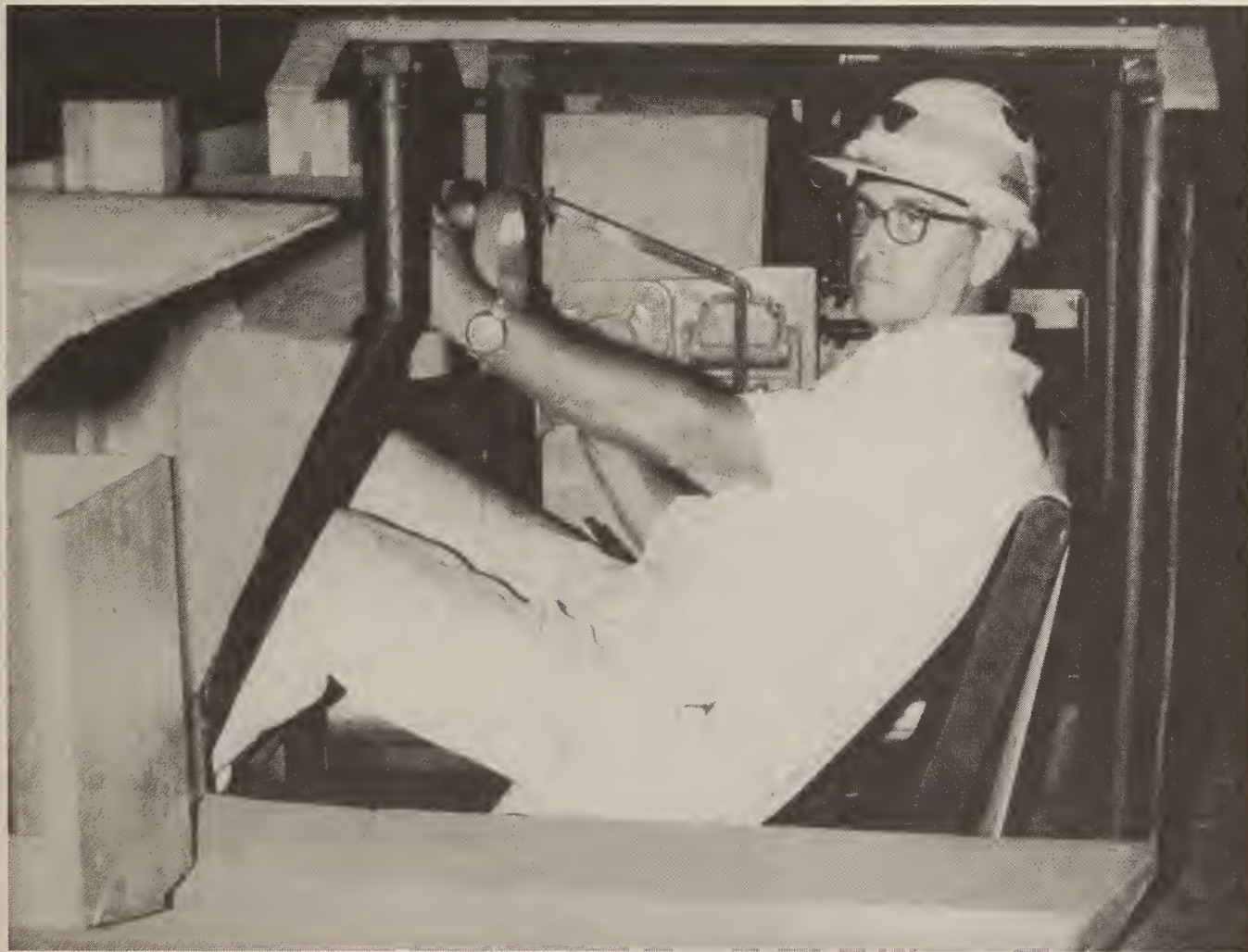
FIGURE 2. - Mockup of transverse-mounted canopy for shuttle car.
