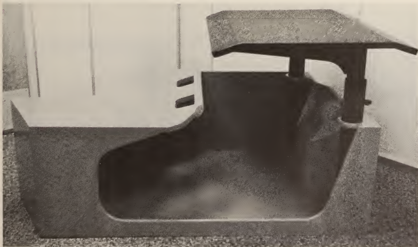
FIGURE 19. - Mockup of two-post cantilevered canopy for cutter and face drill.
