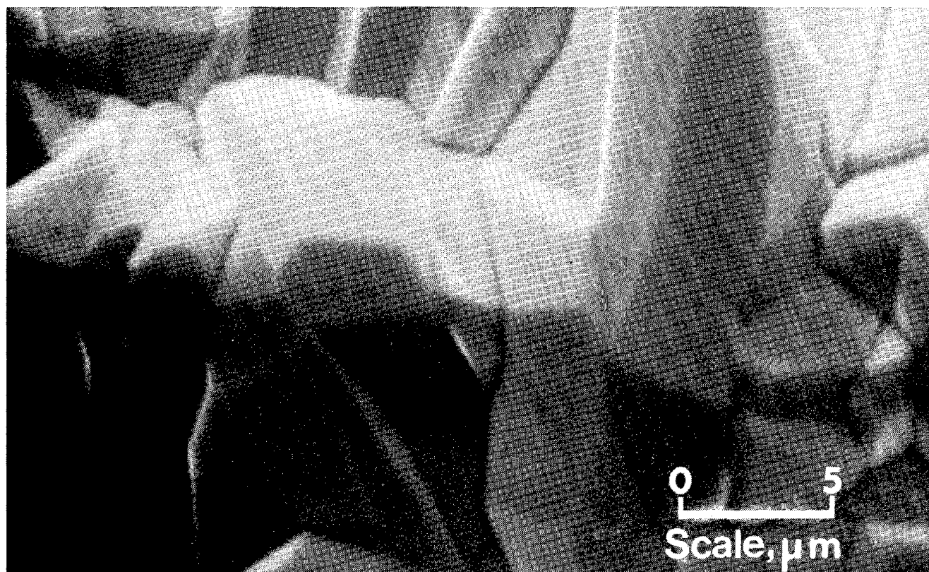
FIGURE 3. • Surface of a direct-current-deposited platinum coating on an Fe-10Cr substrate.
