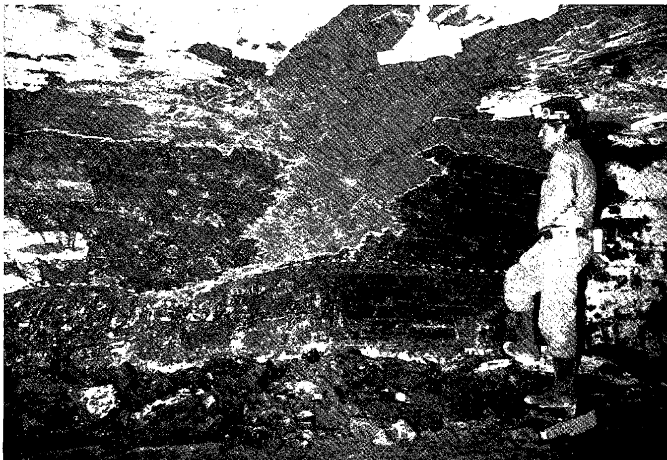
FIGURE 9. - Claystone dike or clay vein transecting coalbed and shale roof.
