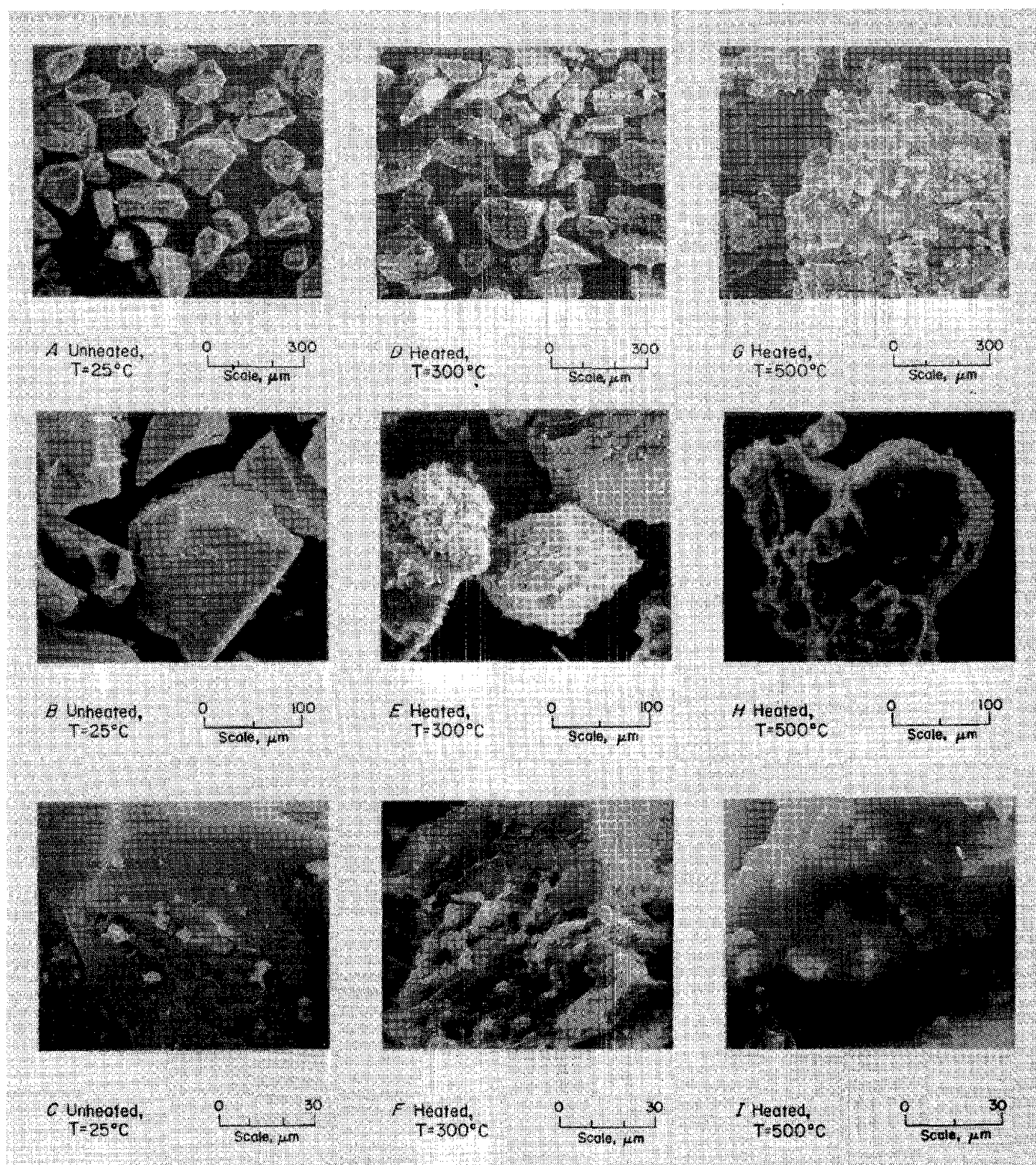
FIGURE 49. - Pittsburgh coal dust slowly heated in a furnace at various temperatures.
