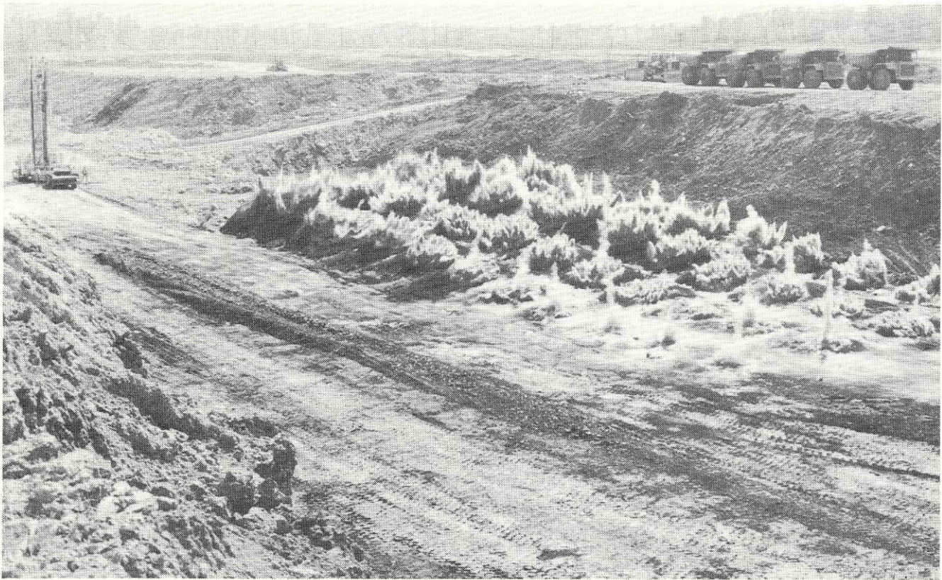
Low-frequency vibrations from surface coal mine production blasts were assessed to develop blast design procedures for vibration control.
