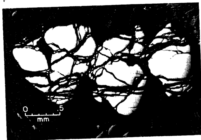
FIGURE 6. - Photomicrograph of polished section showing well-developed lineation defined by alignment of chromite grains and parallel internal fractures.
