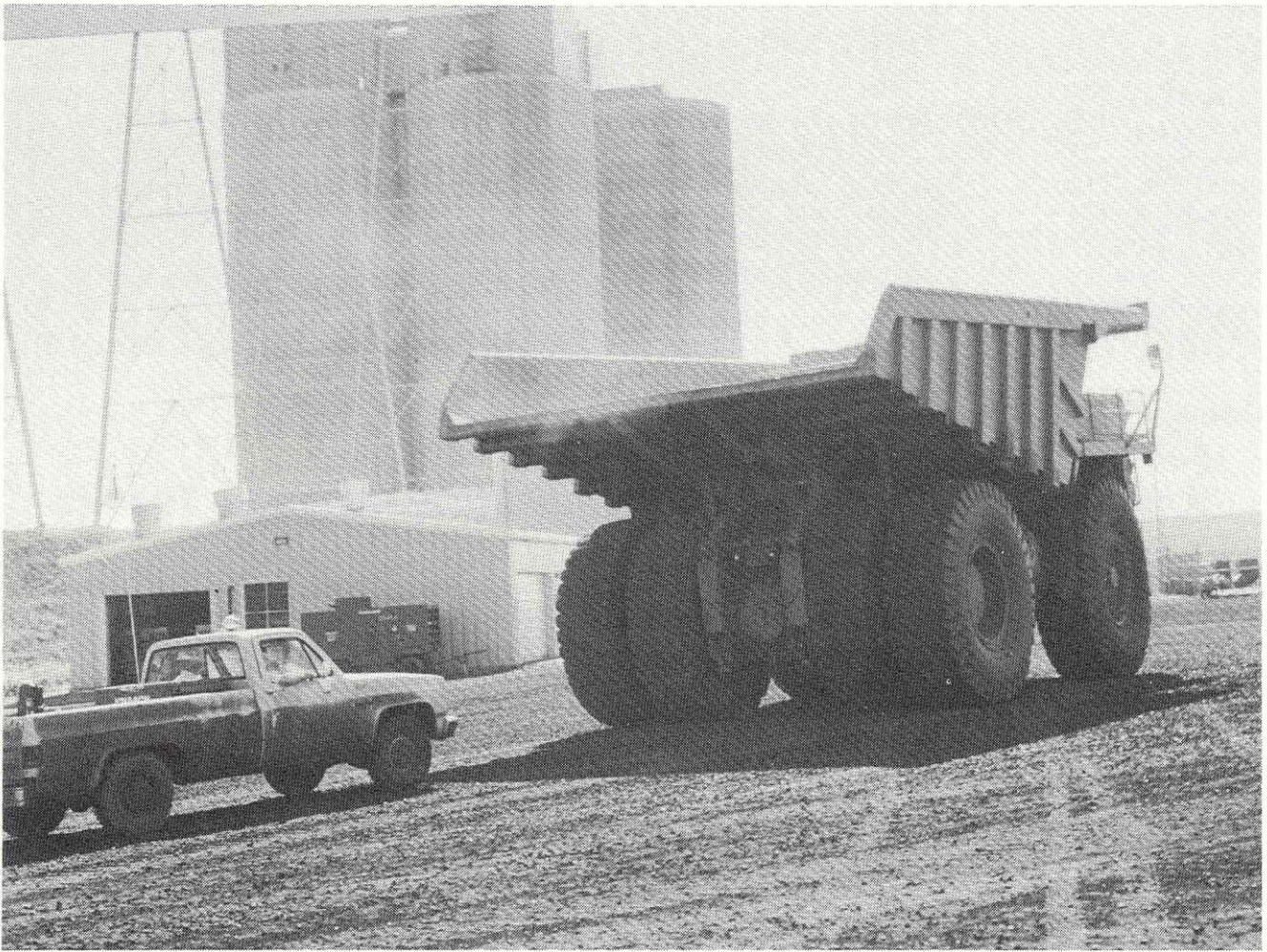
Vehicles in the blind areas of large mine-haulage trucks represent a potential collision hazard if their presence is undetected.
