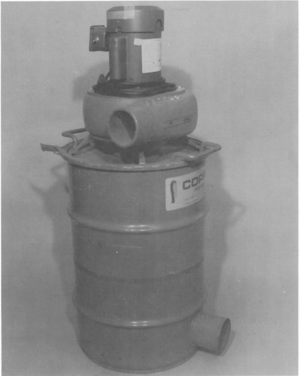
FIGURE 2. - Coppus Portafilter with flexible tubing and nozzle removed. Overall dimensions: 20 by 17 by 40 inches; weight: 77 pounds.
