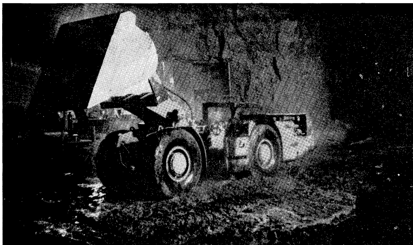
FIGURE A-11. - S.T.3 mucking buggy—used in transporting blasted limestone material out of the drifts.
