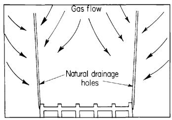
Horizontal boreholes drilled in an active mine are used to drain methane away from the working face.
