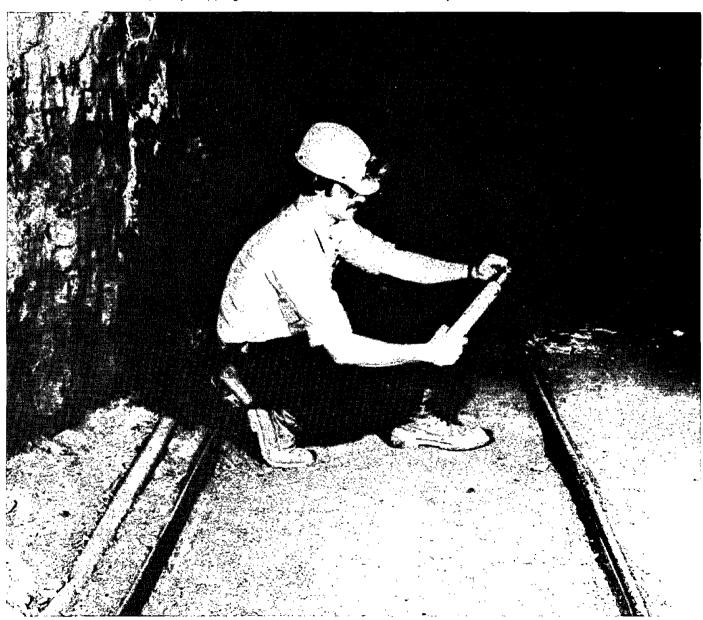
Releasing sulfure hexafluoride (SF<sub>6</sub>), a safe, odorless tracer gas, in a mine airway enables an accurate study of mine ventilation systems.
