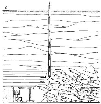
C, when mining passes the borehole, the overlying strata cave in, releasing methane which is drawn out through the borehole instead of into the mine.
