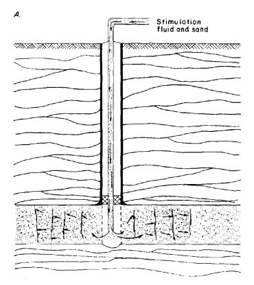
Vertical boreholes to drain methane. A, stimulation fluid and sand are pumped into the coalbed;
