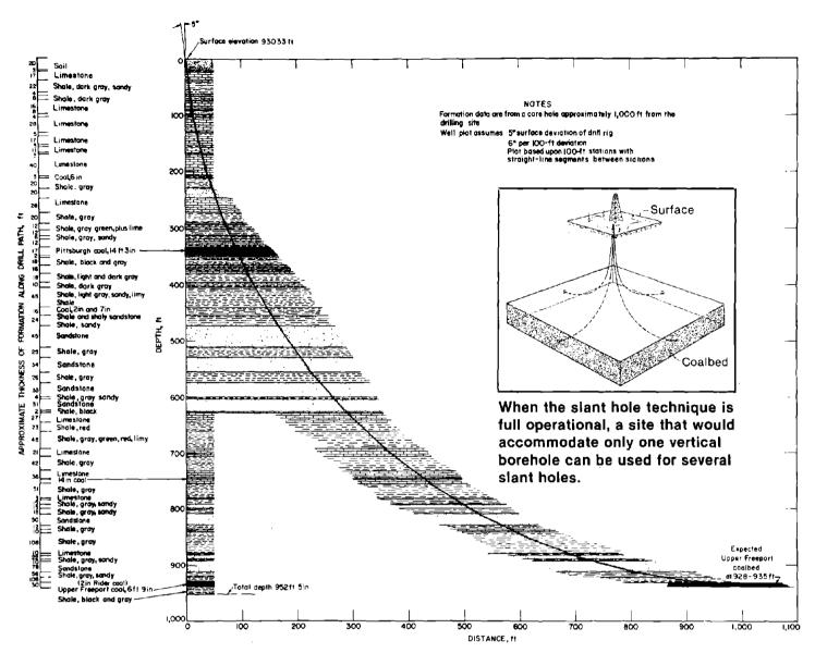
A directional slant hole is drilled from the surface at an angle to intercept the target coalbed horizontally.
