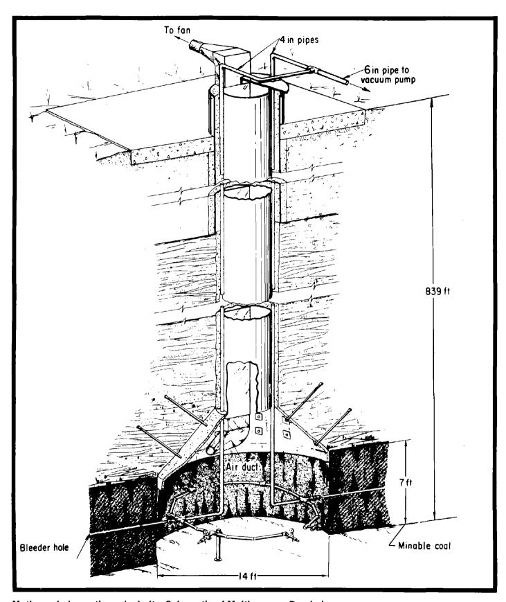
Methane drainage through shafts. Schematic of Multipurpose Borehole.
