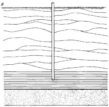
B, a short hole terminates in the strata above the coalbed:
