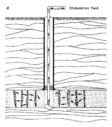
B, stimulation fluid is removed, and sand props open the widened fractures;
