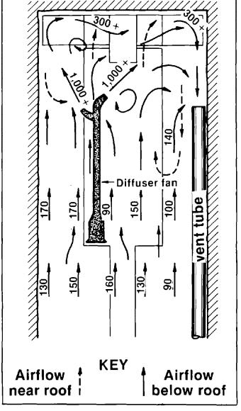
Schematic of the best diffuser fan system for a fullface mining machine.
