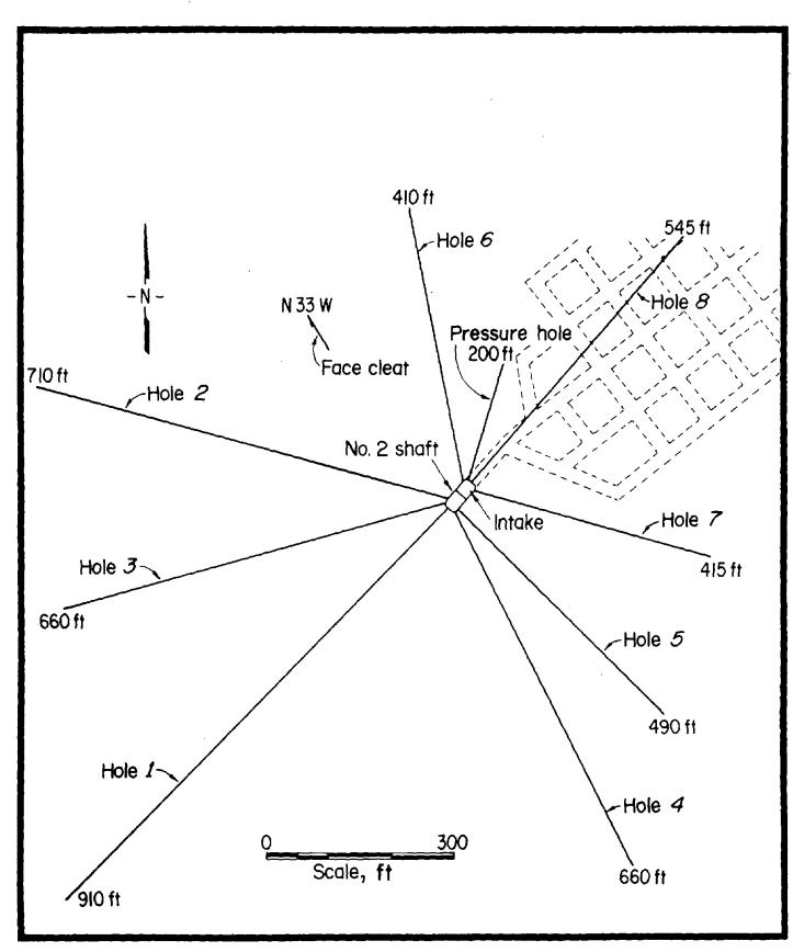
Methane drainage through shafts. Layout of horizontal boreholes and projected mine development at start of drainage project at Multipurpose Borehole.
