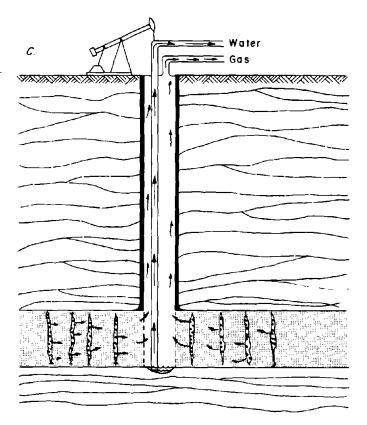
C, gas and water flow from the coalbed.
