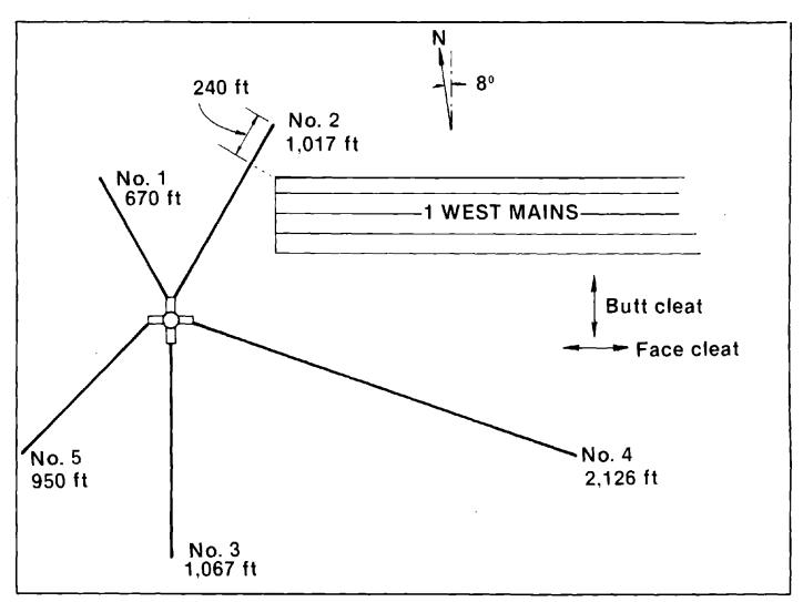
Layout of horizontal boreholes and projected mine development at start of drainage project at Honey Run Shaft.
