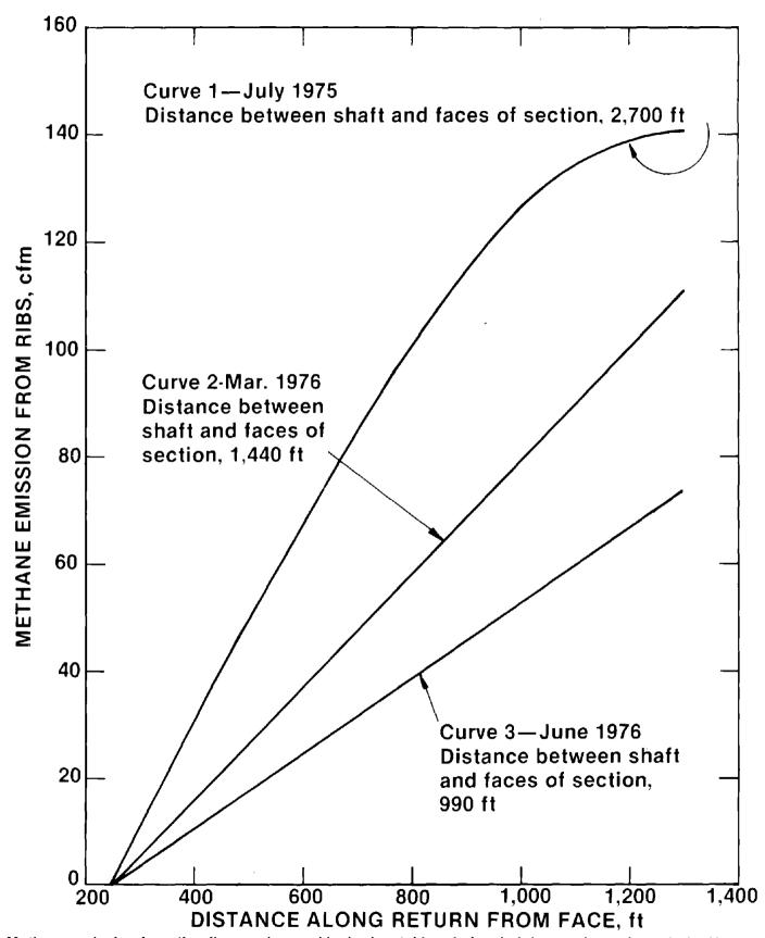
Methane emission from the ribs was lowered by horizontal boreholes draining methane through the Honey Run Shaft.
