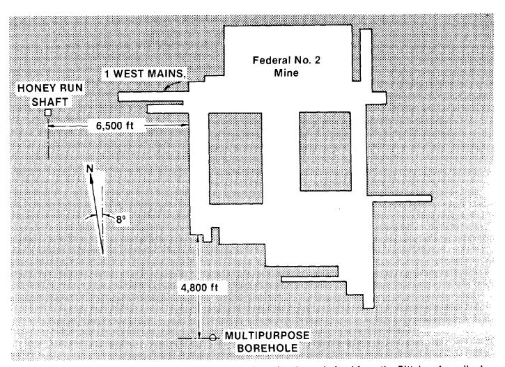
Methane drainage through shafts. Almost 2 Bcf of methane has been drained from the Pittsburgh coalbed through the Multipurpose Borehole and the Honey Run Shaft, both located on the Federal No. 2 Mine property.
