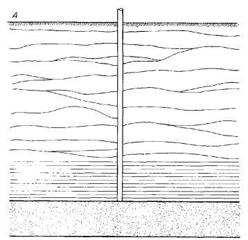
Vertical boreholes for gob ventilation. A, conventional borehole is drilled to the coal before it is mined:
