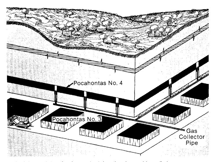
In-mine drainage techniques have been used to drain methane from overlying coalbeds.
