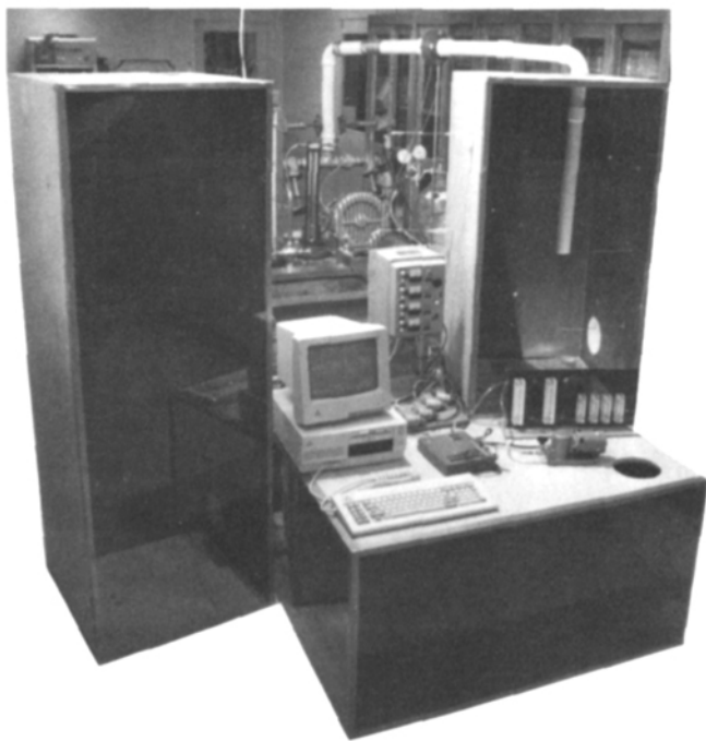
FIGURE 2. Experimental facility showing CS Models C, D, and E (bottom, right, and left, respectively) and the ventilation, nitrogen release, air sampling, and oxygen monitoring systems.
