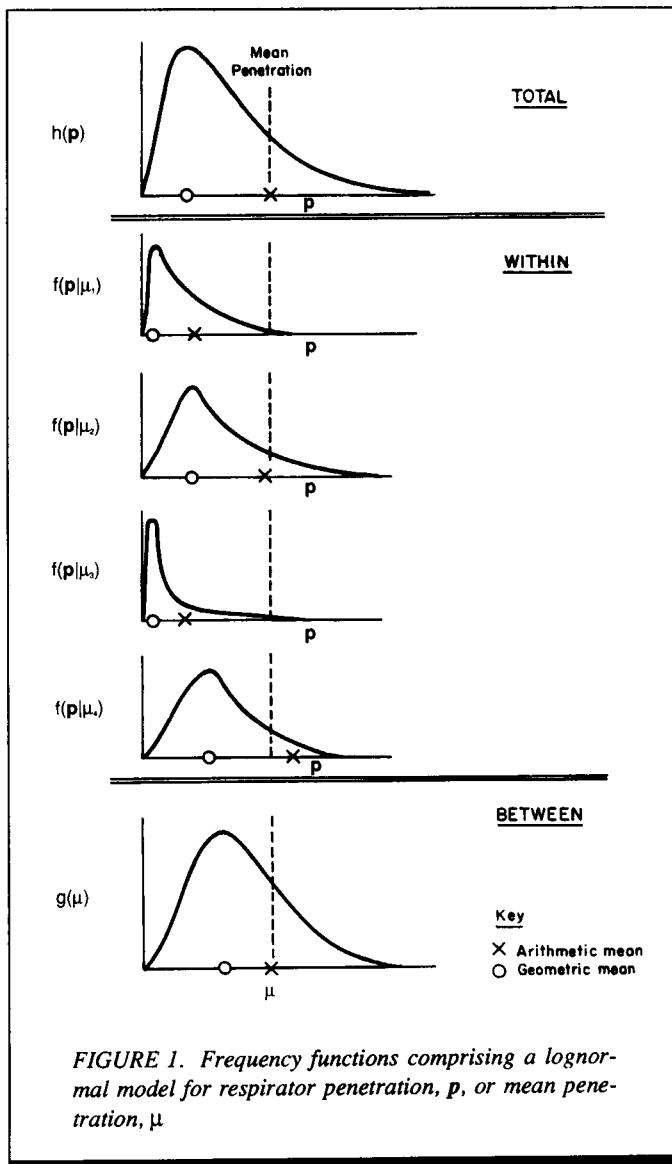
FIGURE 1. Frequency functions comprising a lognormal model for respirator penetration,  $p$ , or mean penetration,  $\mu$
