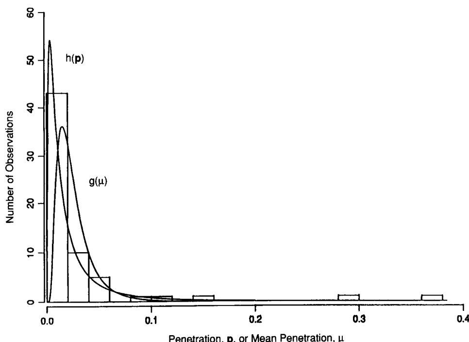
FIGURE 2. Histogram of observed penetration values and the frequency functions  $h(p)$  and  $g(\mu)$  estimated from these data
