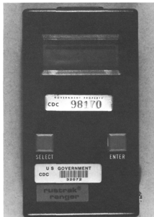
FIGURE 2. Gulton RR-400 Rustrak Ranger data logger.
