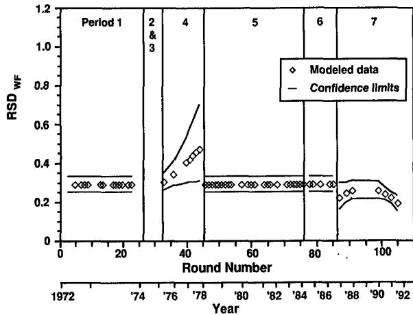
FIGURE 4.  $RSD_{WF}$  model, 300 fibers/mm<sup>2</sup>, chrysotile; 90% confidence limits for all comparisons
