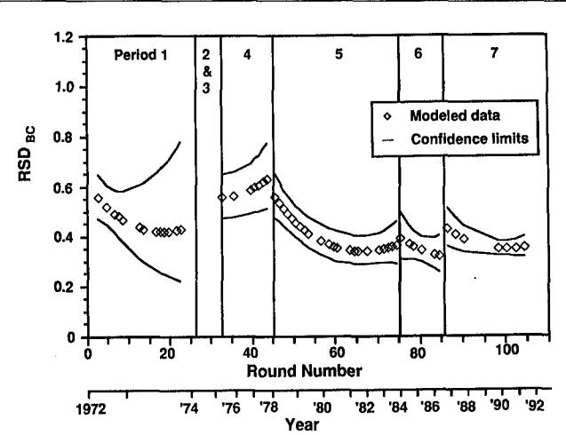
FIGURE 5.  $RSD_{BC}$  model, 300 fibers/mm<sup>2</sup>, chrysotile; 90% confidence limits for all comparisons
