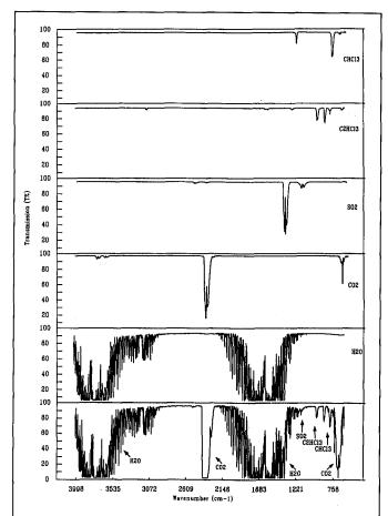
FIGURE 3. Infrared absorption by gases and organic vapors, individually and in a mixture in ambient air.
