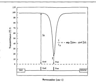
FIGURE 2. Schematic representation of the differential absorption technique in determination of a gas concentration ("c" in the equation on the figure).  $I_O$  and I are the incident and transmitted intensity respectively.  $a_1$  and  $a_2$  are absorption coefficients at  $v_{on}$  and  $v_{off}$  respectively. L is the total path length.
