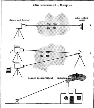
FIGURE 1. Schematic diagram of configurations of remote sensing measurements.
