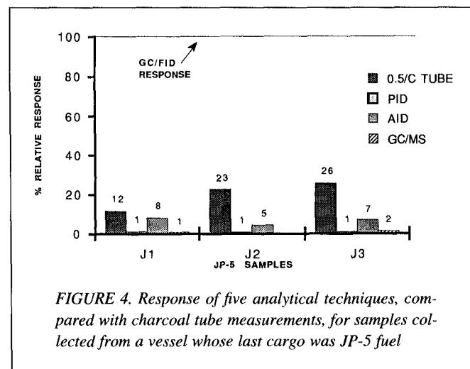
FIGURE 4. Response of five analytical techniques, compared with charcoal tube measurements, for samples collected from a vessel whose last cargo was JP-5 fuel
