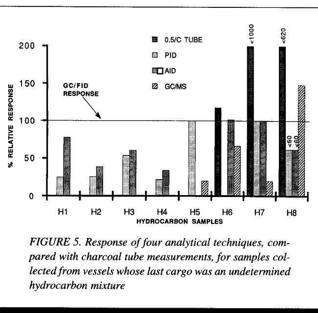
FIGURE 5. Response of four analytical techniques, compared with charcoal tube measurements, for samples collected from vessels whose last cargo was an undetermined hydrocarbon mixture
