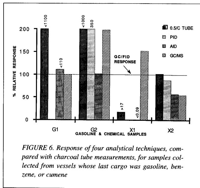
FIGURE 6. Response of four analytical techniques, compared with charcoal tube measurements, for samples collected from vessels whose last cargo was gasoline, benzene, or cumene
