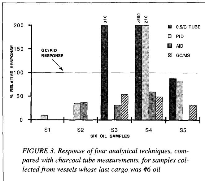
FIGURE 3. Response of four analytical techniques, compared with charcoal tube measurements, for samples collected from vessels whose last cargo was #6 oil
