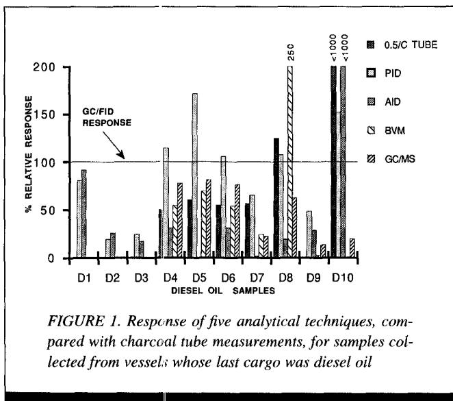
FIGURE 1. Response of five analytical techniques, compared with charcoal tube measurements, for samples collected from vessels whose last cargo was diesel oil
