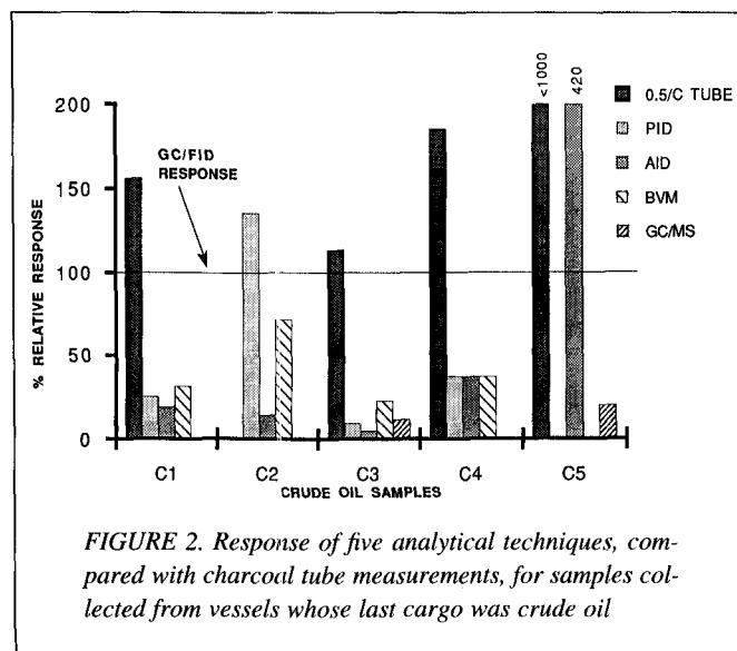
FIGURE 2. Response of five analytical techniques, compared with charcoal tube measurements, for samples collected from vessels whose last cargo was crude oil
