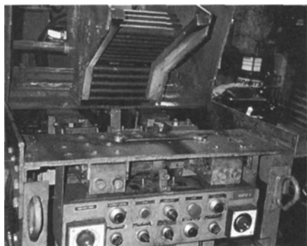
FIGURE 1. Frontal view of ERH device. Note the storage of carbon electrodes.
