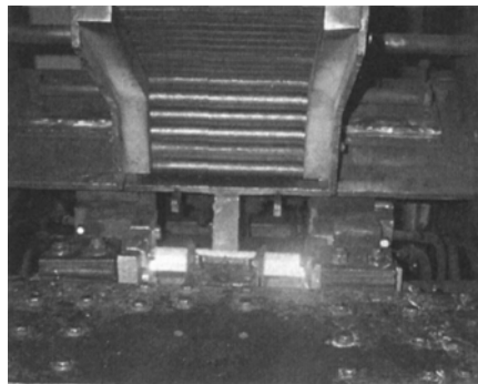
FIGURE 3. Carbon electrode being heated in an ERH.
