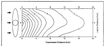
FIGURE 3. Concentration contour map with freestream velocity of 150 fpm at hip level (unit of concentration: ppm)
