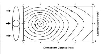
FIGURE 2. Concentration contour map with freestream velocity of 150 fpm at elbow level (unit of concentration: ppm)
