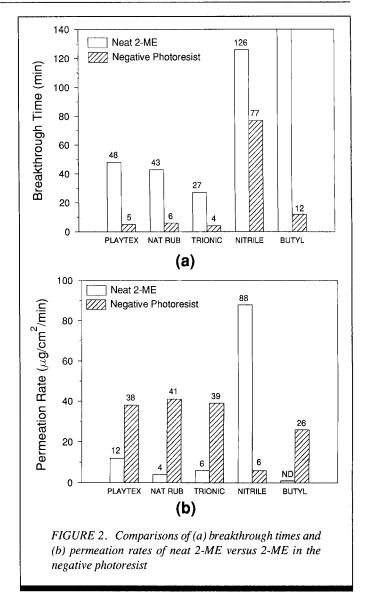
centration is more complex, but the breakthrough time should also decrease as the solvent concentration decreases. For a given solvent/glove pair, the steady-state permeation rate should vary inversely with the thickness of the glove sample. The theoretical variation in breakthrough time with thickness is approximately equal to the ratios of the squares of the thicknesses, as has been observed experimentally.<sup>(33)</sup>
