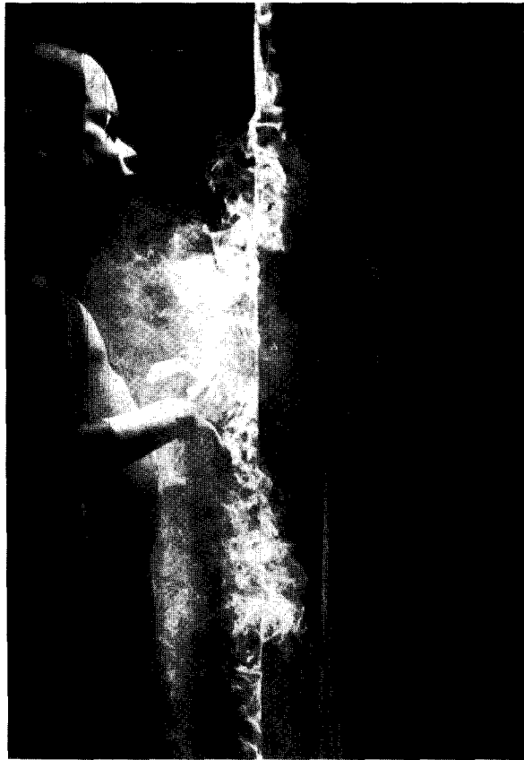
FIGURE 5. Flow visualization for Configuration A side view at 150 ft/min. Smoke wire is between the mannequin and box.
