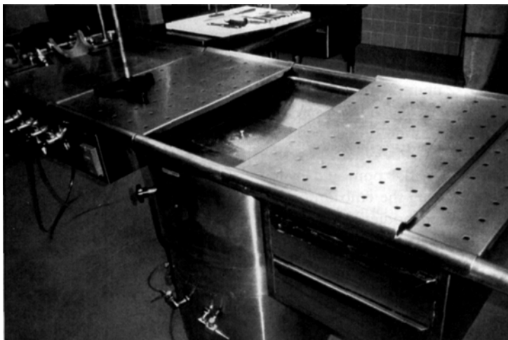
FIGURE 2. Downdraft ventilation table showing the movable perforated drainboard panels and central exhaust with a 10-inch movable perforated strainer.
