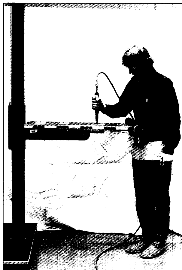
FIGURE 1b. Subject driving screws with an in-line screwdriver at 38 cm with the horizontal surface placed at elbow height.
