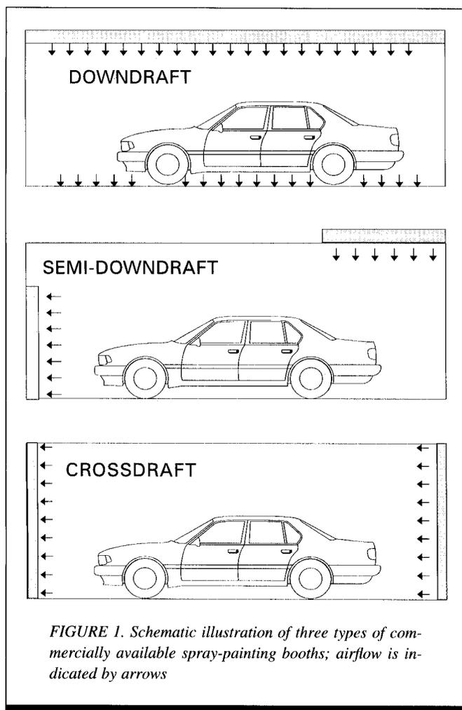
FIGURE 1. Schematic illustration of three types of commercially available spray-painting booths; airflow is indicated by arrows
