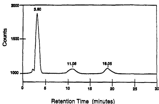
FIGURE 1. HPLC chromatogram of a typical field sample using an electrochemical detector
