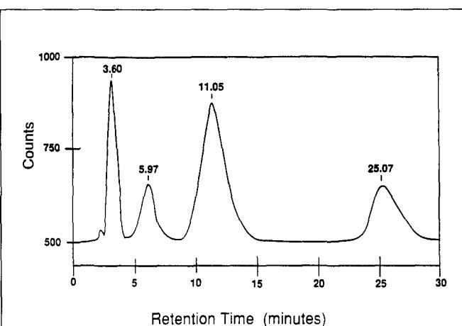
FIGURE 2. HPLC chromatogram of the HDI-containing catalyst bulk sample using an electrochemical detector
