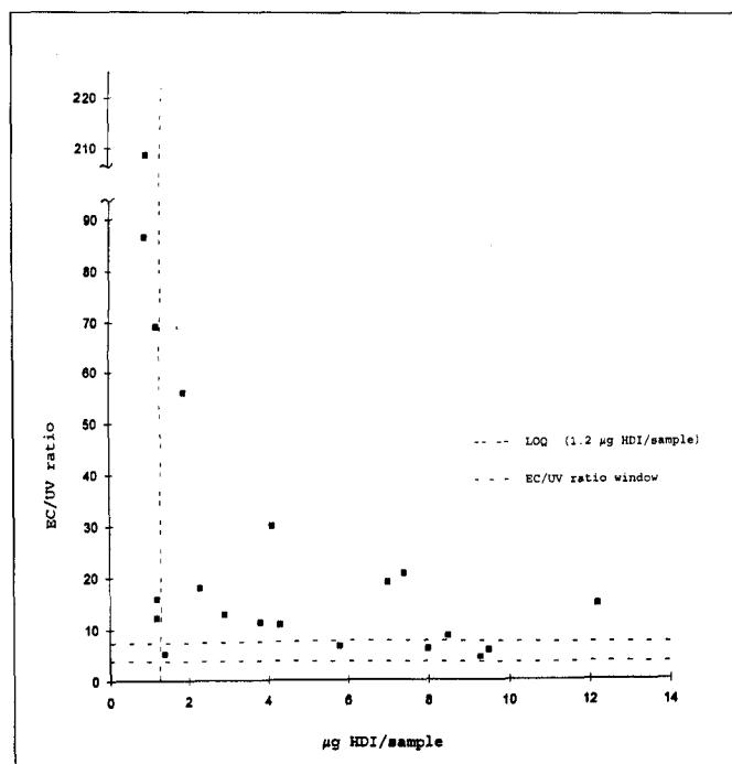
FIGURE 5. Graph of EC/UV detector response versus analyte concentration for the isocyanate-derived peak (11-min retention time) in the field samples
