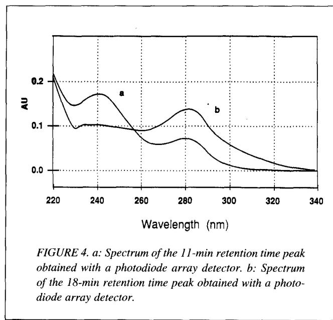
FIGURE 4. a: Spectrum of the 11-min retention time peak obtained with a photodiode array detector. b: Spectrum of the 18-min retention time peak obtained with a photodiode array detector.
