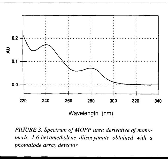
FIGURE 3. Spectrum of MOPP urea derivative of monomeric 1,6-hexamethylene diisocyanate obtained with a photodiode array detector
