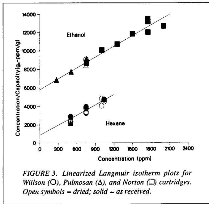
FIGURE 3. Linearized Langmuir isotherm plots for Willson (○), Pulmosan (Δ), and Norton (□) cartridges. Open symbols = dried; solid = as received.
