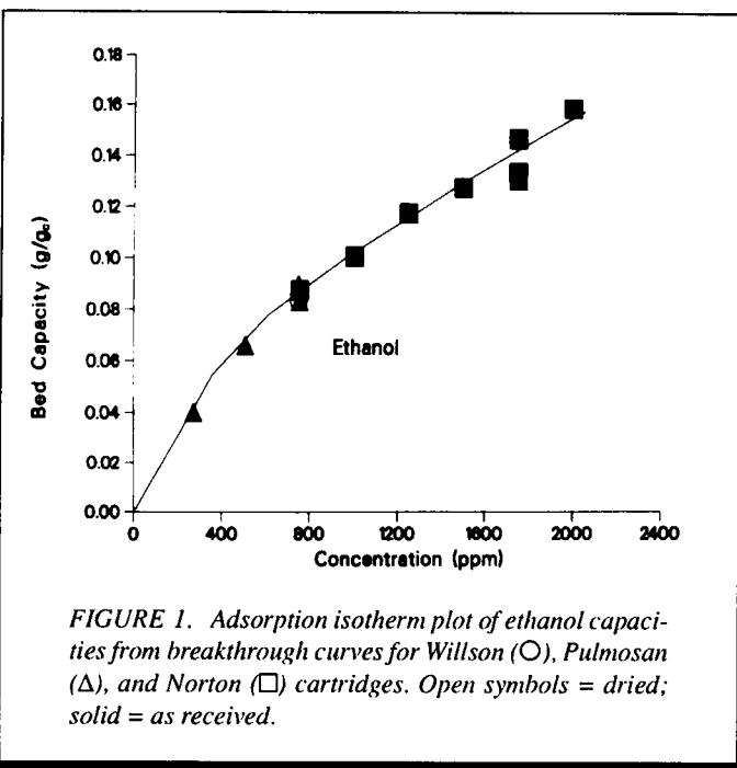
FIGURE 1. Adsorption isotherm plot of ethanol capacities from breakthrough curves for Willson (○), Pulmosan (Δ), and Norton (□) cartridges. Open symbols = dried; solid = as received.
