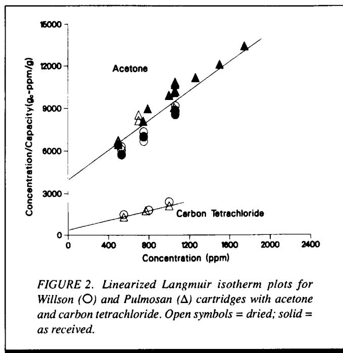
FIGURE 2. Linearized Langmuir isotherm plots for Willson (○) and Pulmosan (Δ) cartridges with acetone and carbon tetrachloride. Open symbols = dried; solid = as received.
