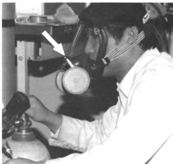
FIGURE 2. A mask with the AESLI in use. The LED location is indicated by the arrow.
